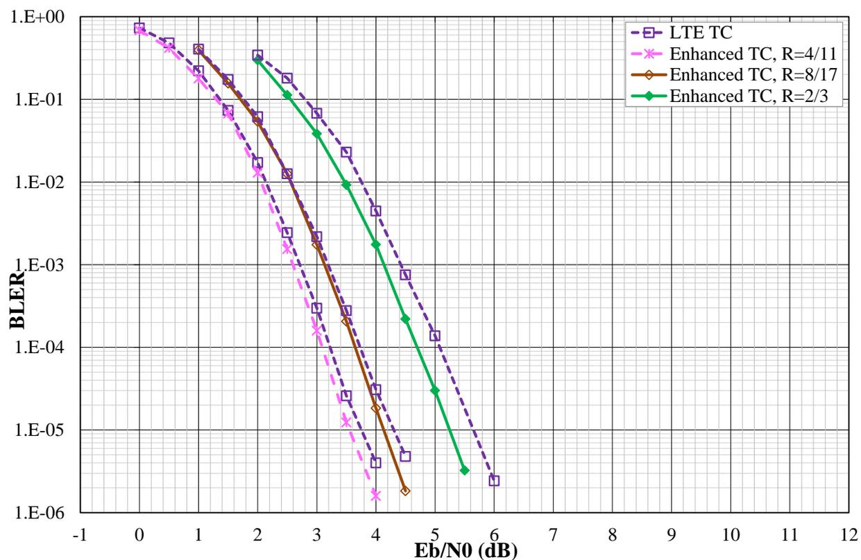
**Figure 9: Performance comparison of the improved turbo code with the LTE turbo code in AWGN channel for coding rates 4/11, 8/17, and 2/3 in terms of Block Error Rate vs Eb/N0. QPSK modulation, block size  $K = 96$  bits, 8 decoding iterations of the Max-Log-MAP algorithm, tail-biting termination.**
