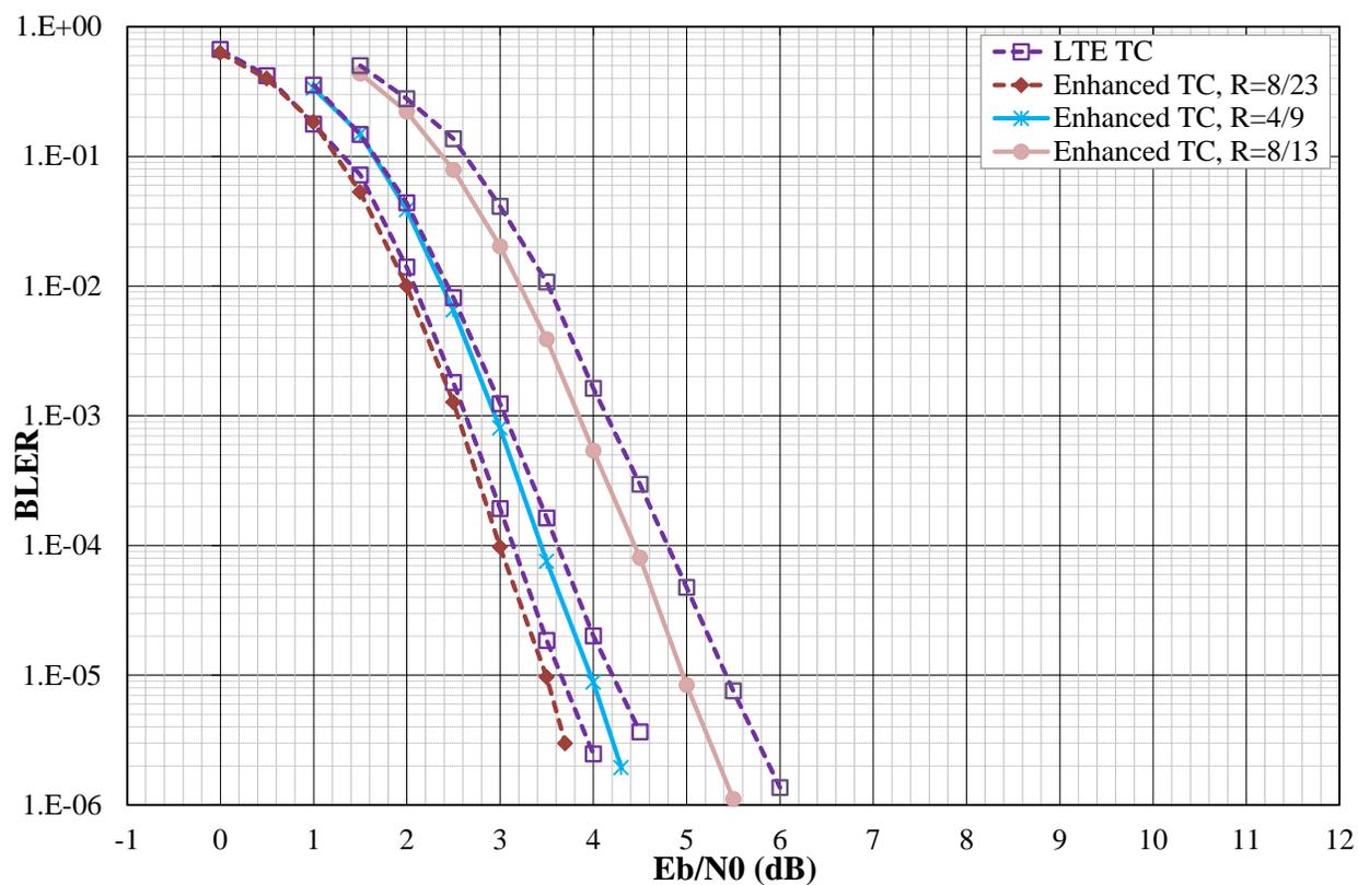
**Figure 8: Performance comparison of the improved turbo code with the LTE turbo code in AWGN channel for coding rates 8/23, 4/9, and 8/13 in terms of Block Error Rate vs Eb/N0. QPSK modulation, block size  $K = 96$  bits, 8 decoding iterations of the Max-Log-MAP algorithm, tail-biting termination.**
