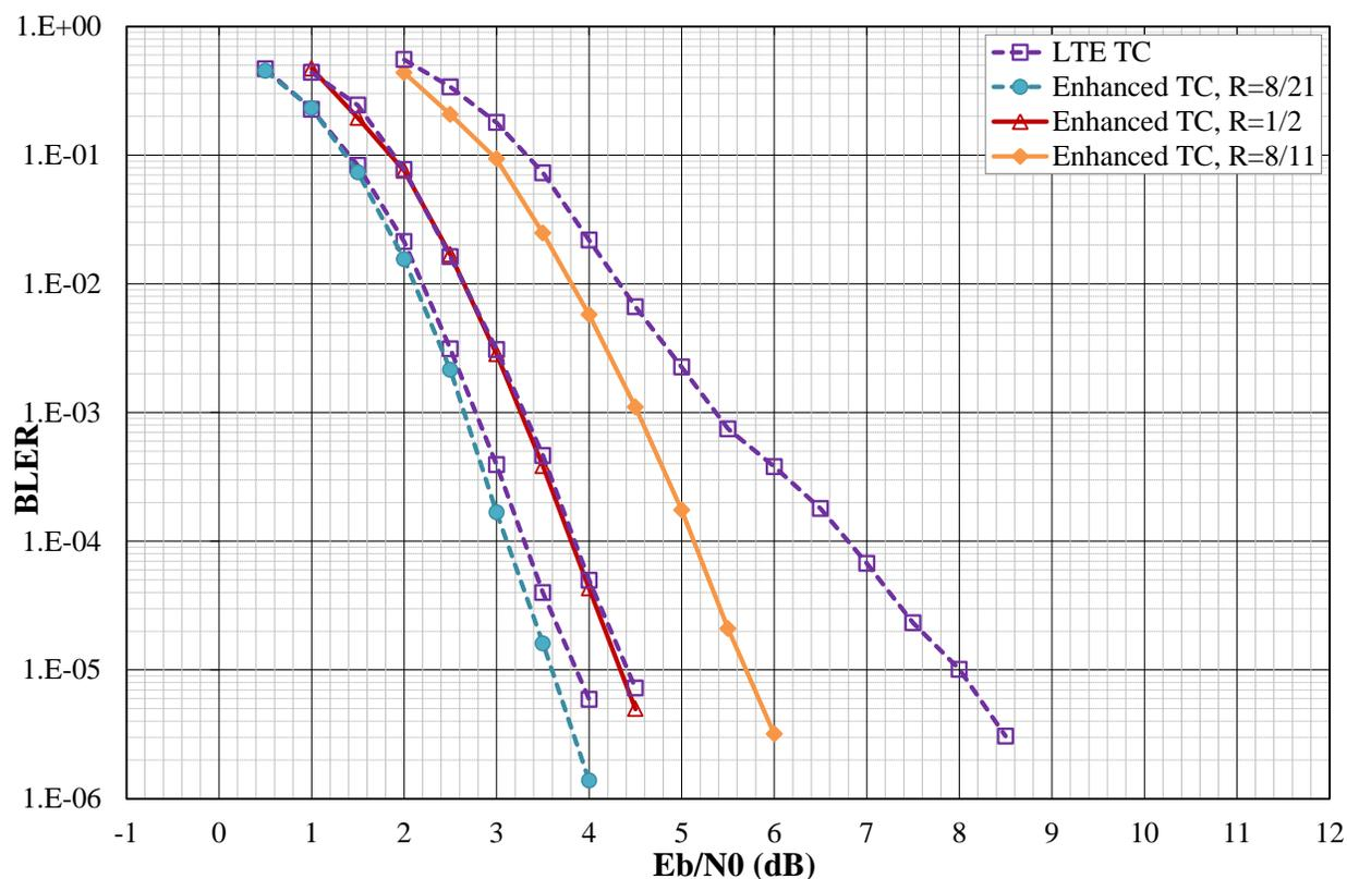
**Figure 10: Performance comparison of the improved turbo code with the LTE turbo code in AWGN channel for coding rates 8/21, 1/2, and 8/11 in terms of Block Error Rate vs Eb/N0. QPSK modulation, block size  $K = 96$  bits, 8 decoding iterations of the Max-Log-MAP algorithm, tail-biting termination.**
