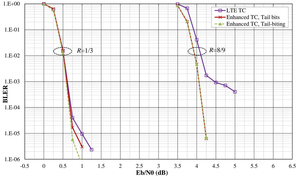
**Figure 3: Performance comparison of the improved turbo code (when using tail bits or tail-biting termination) with the LTE turbo code in AWGN channel for coding rates 1/3 and 8/9 in terms of Block Error Rate vs Eb/N0.**
