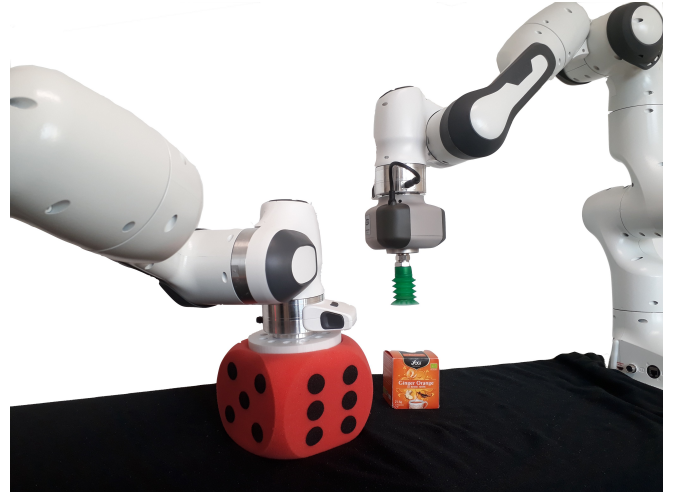
Fig. 1: Panda manipulators equipped with a rigid flat end-effector (left) and with a pump plus flexible suction cup (right). In the experiments, we identify the deformation dynamics for the soft dice (left) and the sucker (right) in order to initiate contacts with the maximum allowed impact.
