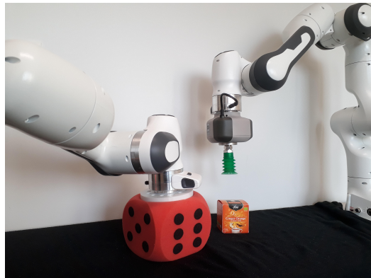
Fig. 1: Panda manipulators equipped with a rigid flat end-effector (left) and with a pump plus flexible suction cup (right). In the experiments, we identify the deformation dynamics for the soft dice (left) and the sucker (right) in order to generate maximum impact.
