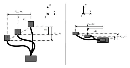
Figure 18: 3D displacement test illustrative scheme seen from camera 1's point of view (left) and from above (right).
