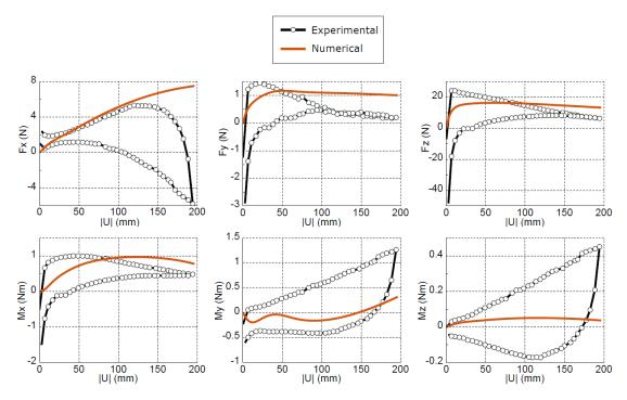
Figure 21: 6 reaction forces and torques during loading for the experiment and the real Timoshenko model - sample 1.
