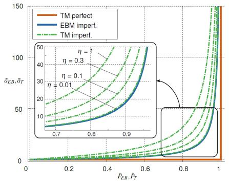
(b) TM axial load vs. transverse displacement equilibrium curves for several values of the shearing parameter  $\eta$  and a fixed initial deflection  $\bar{a}_0=2$ . The result is compared to the EBM equilibrium curve with the same  $\bar{a}_0$ .
