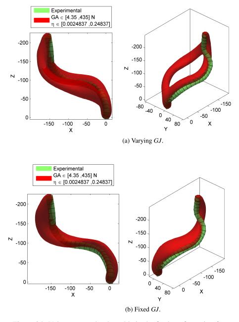
Figure 24: Volume swept by the cable in the final configuration for a varying GA - sample 1.
