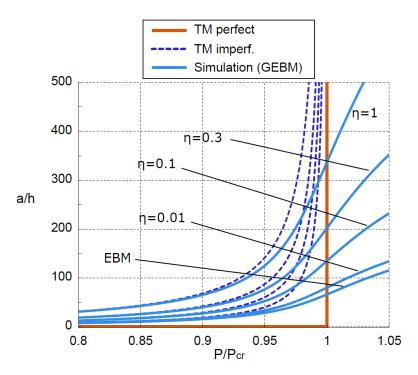
Figure 9: Normalized equilibrium curves for the simulation [Cottanceau et al., 2018] based on a geometrically exact beam model (TM). The results are presented for several values of  $\eta$  and compared to the 2<sup>nd</sup> order TM buckling theory.
