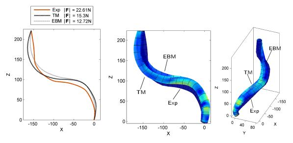
Figure 22: 3D displacement test - Final deformed shapes of sample 1 with TM, EBM vs. experimental deformed shape.
