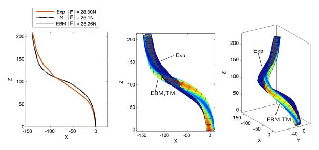
Figure 23: 3D displacement test - Final deformed shapes of sample 3 with TM, EBM vs. experimental deformed shape.
