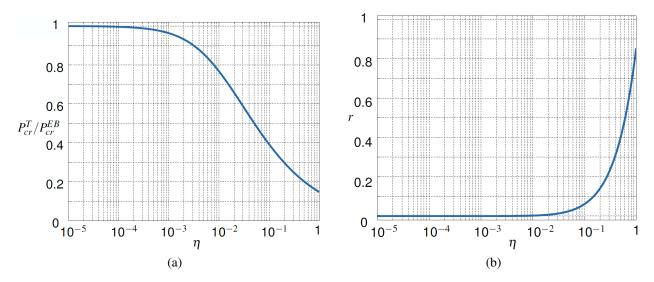
Figure 7: Influence of the shearing on the critical force: (a) ratio of the TM critical force to the EBM critical force as a function of the shearing parameter  $\eta$ ; (b) ratio of the partial derivatives with respect to  $GAL^2$  and EI,  $r = \left| \frac{\partial P_{\text{cr}}^{\text{T}}/\partial (GAL^2)}{\partial P_{\text{cr}}^{\text{T}}/\partial (EI)} \right|$ , as a function of  $\eta$ .
