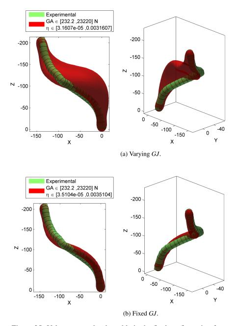
Figure 25: Volume swept by the cable in the final configuration for a varying GA - sample 3.
