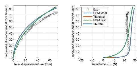
Figure 14: Post-buckling test - Equilibrium curves for sample 2 (large identified *GA*): transverse displacement of the beam middle vs. axial displacement (left) and axial force (right).
