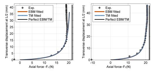
Figure 13: Identification curves on the buckling test for samples 4 and 5.
