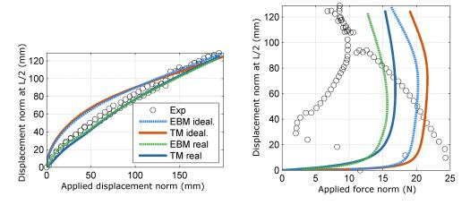
Figure 19: 3D displacement test - Equilibrium curves for sample 1: transverse displacement at beam middle vs. axial displacement (left) and axial force (right).
