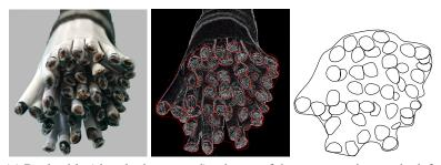
(a) Real cable (signal wires strand): picture of the cross-section on the left; approximate reconstruction of the real cable cross-section (middle and right).
