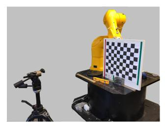
Figure 4: Illustration of the calibration of camera 2 with a checkerboard.
