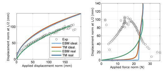
Figure 20: 3D displacement test - Equilibrium curves for sample 3: transverse displacement at beam middle vs. axial displacement (left) and axial force (right).
