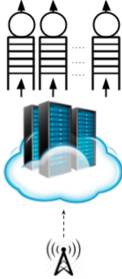
Figure 1: Fog node processing in parallel queues
