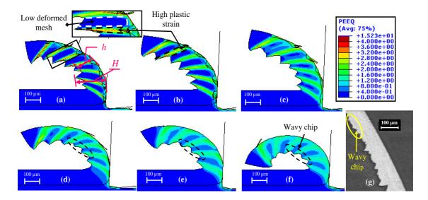
**Fig. 13** Comparison of the numerical chip predicted with different FE edge lengths ((a) 4  $\mu$ m, (b) 6  $\mu$ m, (c) 8  $\mu$ m, (d) 10  $\mu$ m, (e) 12  $\mu$ m and (f) 14  $\mu$ m) to (g) the experimental one (Calamaz, 2008) ( $V_c = 33$  m/min and f = 0.1 mm/rev)
