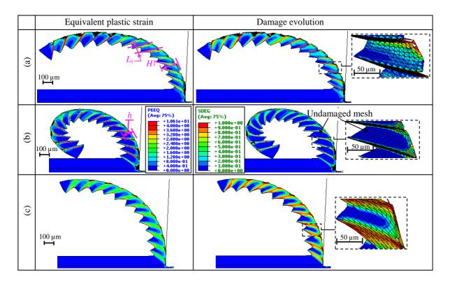
Fig. 19 Chip morphology, plastic strains and damage evolution corresponding to different meshing methods: (a) 1, (b) 2 and (c) 3 ( $V_c = 75$  m/min)
