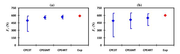
**Fig. 22** Comparison of computed cutting forces to the experimental ones of the literature (Calamaz et al., 2010): (a) 33 m/min and (b) 75 m/min
