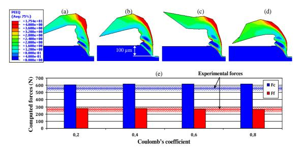
**Fig. 12** Sensitivity of (a-d) the chip morphology and (e) computed forces to the friction coefficient: (a)  $\mu = 0.2$ , (b)  $\mu = 0.4$ , (c)  $\mu = 0.6$  and (d)  $\mu = 0.8$  (*ALE-Lag* FE model,  $V_c = 75$  m/min and  $G_f = 18$  N/mm)
