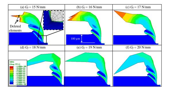
Fig. 7 Effect of failure energy on the chip morphology modeled with the *ALE-Lag* approach  $(V_c = 75 \text{ m/min}, f = 0.1 \text{ mm/rev and } \mu = 0.1)$
