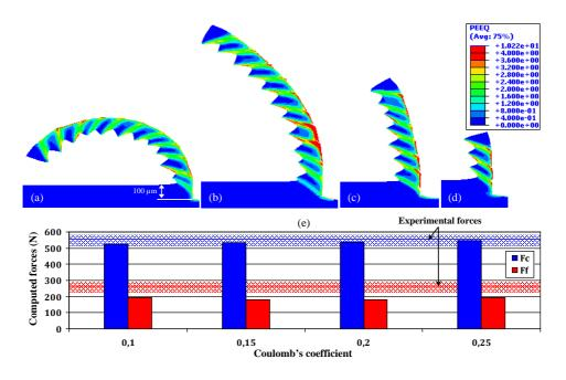
**Fig. 11** Effect of the friction coefficient on the numerical chip morphology ((a)  $\mu = 0.1 \_ t_c = 1$  ms, (b)  $\mu = 0.15 \_ t_c = 0.61$  ms, (c)  $\mu = 0.2 \_ t_c = 0.41$  ms and (d)  $\mu = 0.25 \_ t_c = 0.31$  ms) and (e) the computed forces ( $V_c = 75$ /min and  $G_f = 15$  N/mm)
