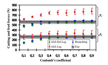
**Fig. 5** Comparison of computed forces with the experimental ones of Calamaz et al. (Calamaz et al., 2010) ( $V_c = 75 \text{ m/min}, f = 0.1 \text{ mm/rev}$  and  $a_p = 3 \text{ mm}$ )
