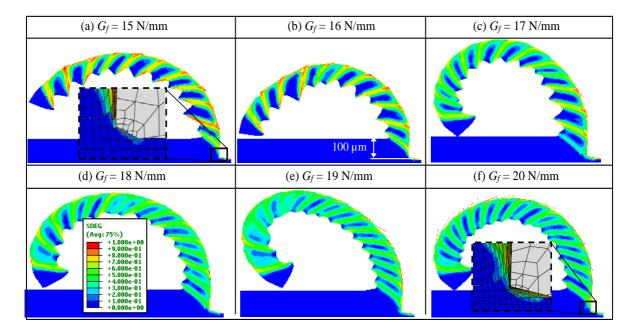
**Fig. 6** Sensitivity of the chip morphology predicted with the *pure Lag* meshing approach to the failure energy ( $V_c = 75 \text{ m/min}, f = 0.1 \text{ mm/rev}$  and  $\mu = 0.1$ )
