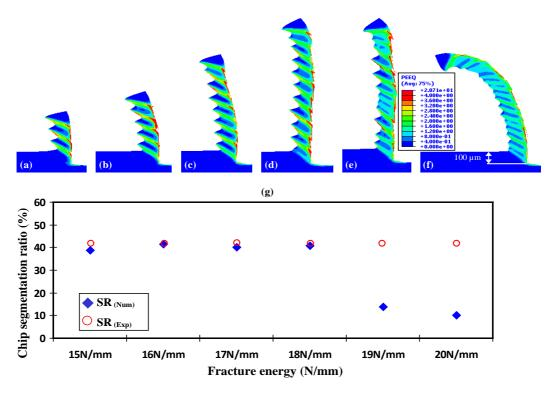
**Fig. 10** Effect of the failure energy on the chip serration ((a)  $G_f = 15$  N/mm, (b)  $G_f = 16$  N/mm, (c)  $G_f = 17$  N/mm, (d)  $G_f = 18$  N/mm, (e)  $G_f = 19$  N/mm and (f)  $G_f = 20$  N/mm) and (g) the segmentation ratio ( $V_c = 75$  m/min and  $\mu = 0.25$ )
