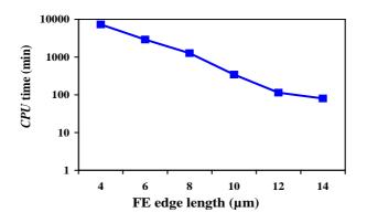
Fig. 17 Computing time as a function of the mesh size ( $V_c = 75$  m/min)
