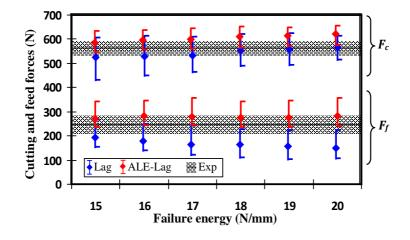
Fig. 9 Effect of failure energy and FE meshing approaches on the computed forces  $(V_c = 75 \text{ m/min}, f = 0.1 \text{ mm/rev and } \mu = 0.1)$
