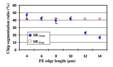
Fig. 15 Numerical chip segmentation ratio sensitivity to the FE edge lengths  $(V_c = 75 \text{ m/min})$
