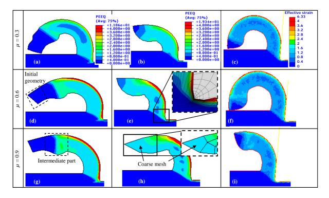
**Fig. 4** Chip morphology predicted with different adaptive meshing approaches ((a, d and g) the *ALE-Eul-Lag* model, (b, e and h) the *ALE-Lag* model and (c, f and i) the remeshing model) and several friction coefficients ((a-c)  $\mu = 0.3$ , (d-f)  $\mu = 0.6$  and (g-i)  $\mu = 0.9$ )
