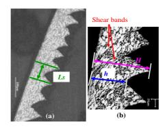
Fig. 3 Experimental chip morphology (Calamaz, 2008) ( $V_c = 75 \text{ m/min} \_ f = 0,1 \text{ mm/rev}$ )
