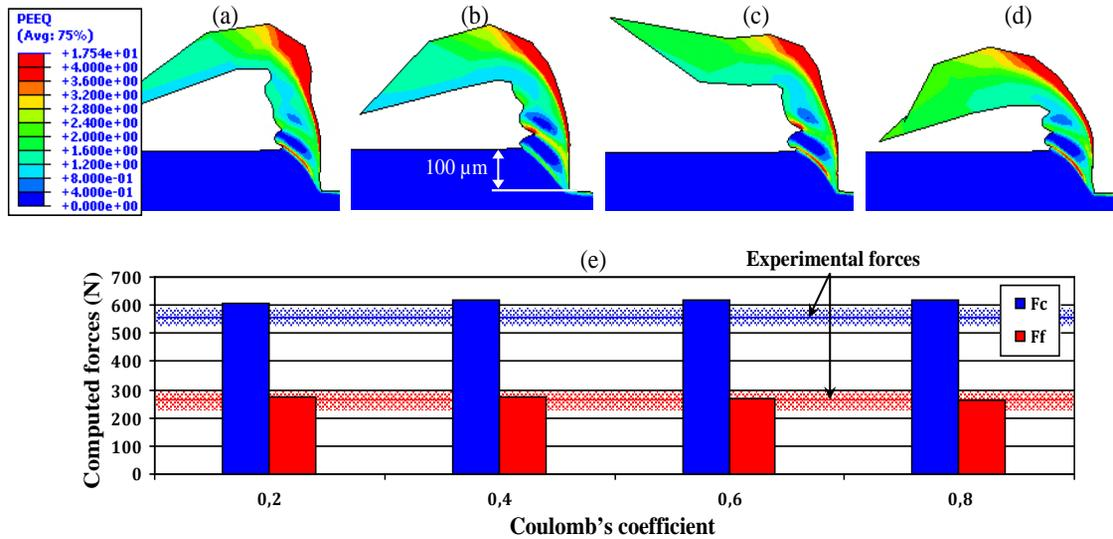
**Fig. 12** Sensitivity of (a-d) the chip morphology and (e) computed forces to the friction coefficient: (a)  $\mu = 0.2$ , (b)  $\mu = 0.4$ , (c)  $\mu = 0.6$  and (d)  $\mu = 0.8$  (*ALE-Lag* FE model,  $V_c = 75$  m/min and  $G_f = 18$  N/mm)
