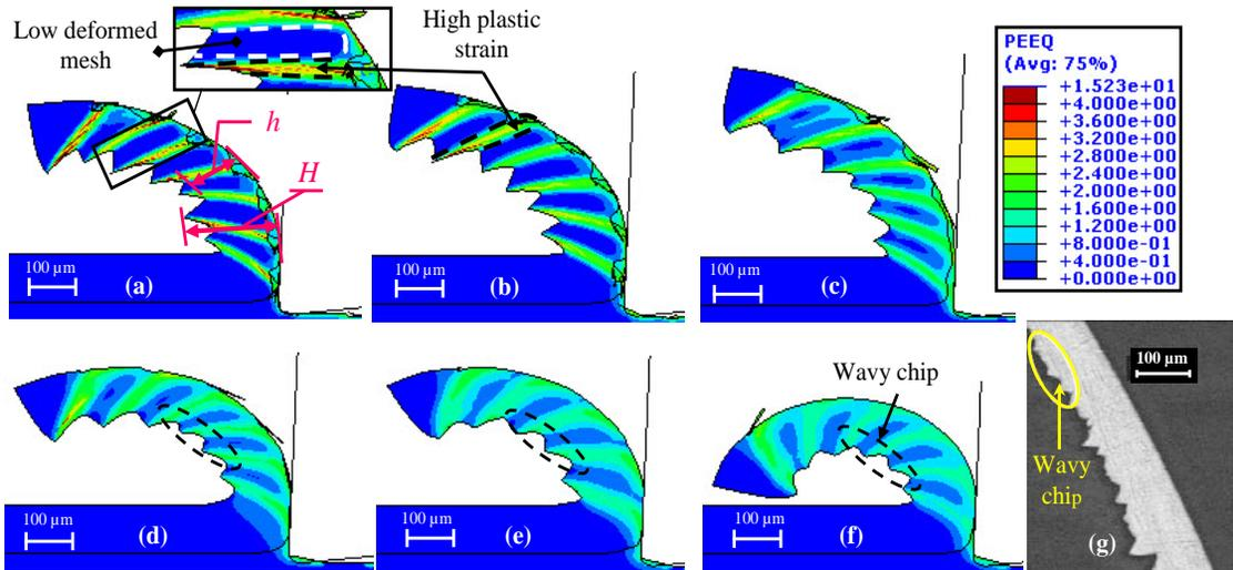
**Fig. 13** Comparison of the numerical chip predicted with different FE edge lengths ((a) 4  $\mu\text{m}$ , (b) 6  $\mu\text{m}$ , (c) 8  $\mu\text{m}$ , (d) 10  $\mu\text{m}$ , (e) 12  $\mu\text{m}$  and (f) 14  $\mu\text{m}$ ) to (g) the experimental one (Calamaz, 2008) ( $V_c = 33$  m/min and  $f = 0.1$  mm/rev)
