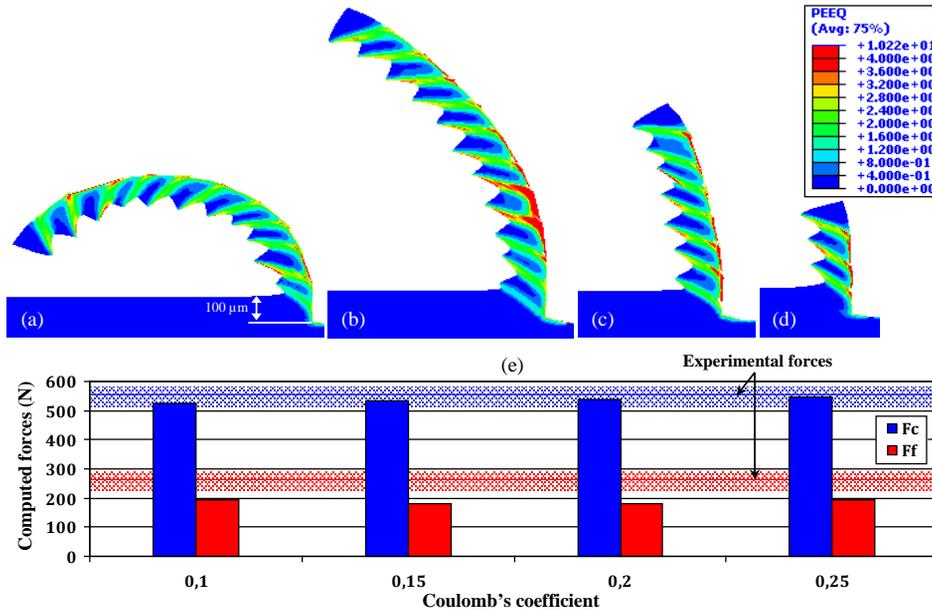
**Fig. 11** Effect of the friction coefficient on the numerical chip morphology ((a)  $\mu = 0.1$  \_  $t_c = 1$  ms, (b)  $\mu = 0.15$  \_  $t_c = 0.61$  ms, (c)  $\mu = 0.2$  \_  $t_c = 0.41$  ms and (d)  $\mu = 0.25$  \_  $t_c = 0.31$  ms) and (e) the computed forces ( $V_c = 75/\text{min}$  and  $G_f = 15$  N/mm)
