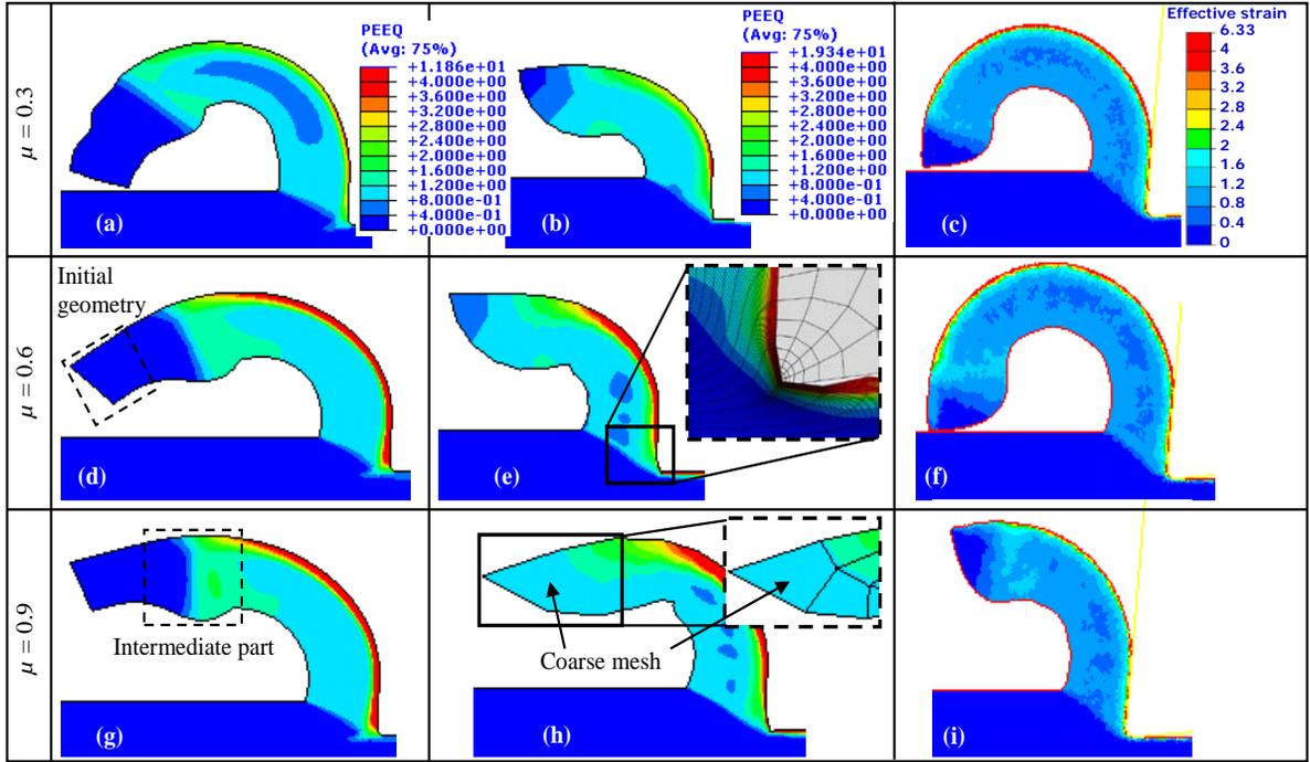
**Fig. 4** Chip morphology predicted with different adaptive meshing approaches ((a, d and g) the *ALE-Eul-Lag* model, (b, e and h) the *ALE-Lag* model and (c, f and i) the remeshing model) and several friction coefficients ((a-c)  $\mu = 0.3$ , (d-f)  $\mu = 0.6$  and (g-i)  $\mu = 0.9$ )
