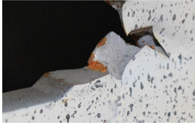
Fig. 8: Crack bifurcation in CT specimen with positive with positive T-stress-induced crack curving T/K= + 2.05 X_{ef} = 0.49 \text{ mm}
