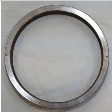
Fig 4: Ring Drop Weight Test (RDWT) specimen
