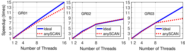
Fig. 13. Speed up factors of anySCAN and an ideal algorithm w.r.t. different numbers of threads
