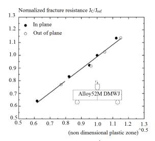
Fig. 9: Normalized fracture resistance  $J_C/J_{ref}$  versus  $\sqrt{A_p}$  for cracked dissimilar metal welded joints, obtained from  $\varepsilon_p = 1.0$  isolines [38].
