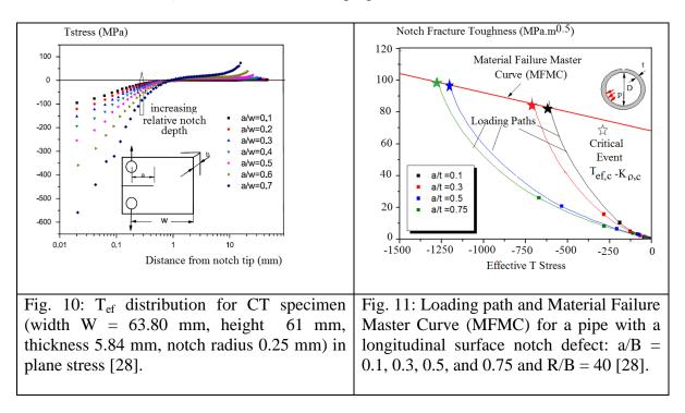
One notes that the value of  $T_{ef}$  increases when a/W increases. This result is confirmed by [41], where T,Q,  $\beta$ , and A<sub>2</sub> are computed for a clamped single-edge tension specimen. The relative crack depth varies in the range a/W = 0.3–0.7 at the loading level of J/(b $\sigma_0$ ) = 0.01, where b is the ligament size. These authors indicate that, in general, T, –Q,  $\beta$ , and –A<sub>2</sub> increase as a/W increases; however, the impact of a/W is relatively small.
