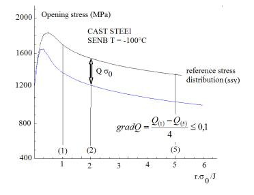
Fig. 6. Definition of Q parameter and validity condition.
