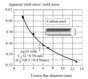
Fig. 21. Applications of Malmberg [22] to bars in torsion.
