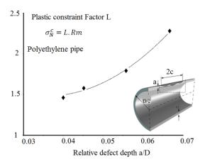
Fig. 7: Evolution of the plastic constraint factor versus the relative defect depth a/D. Polyethylene pipe.
