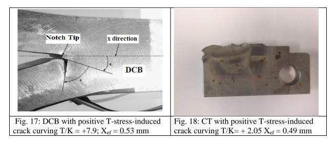
For negative T stress, after initiation, the crack propagates firstly in an instable manner and secondly after several millimetres in a stable manner. During crack propagation in a stable manner, crack tip opening angle CTOA remains constant and its constant value is a characteristic of the fracture resistance of the material. It can be noted that during the stable crack propagation both CTOA and T stress are constant.
