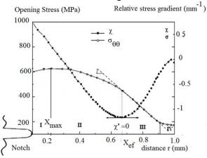
Figure 3 : Elastic-plastic stress distribution and definition of the effective distance from the minimum of the relative stress gradient.
