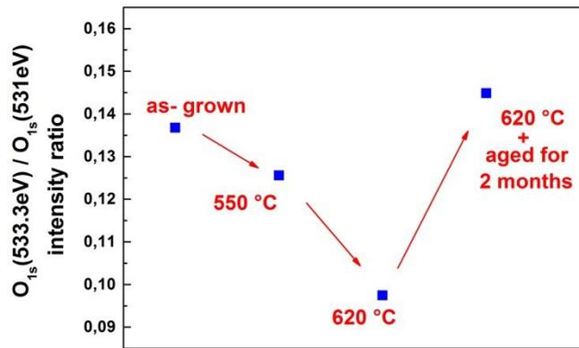
**Figure 5** Intensity ratio between (533.3 eV)- and (531 eV)- O<sub>1s</sub> peaks for the different treated samples
