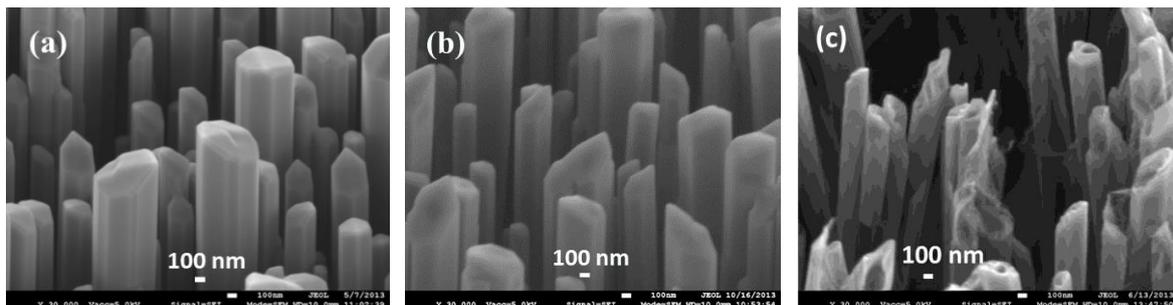
**Figure 2** SEM images of ZnO nanowires
