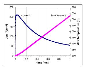
Figure IV-1: Current density and the maximum temperature inside the device versus time during a 500V/1ms  $V_{DS}$ -ramp. (channel depth=0,2  $\mu$ m; channel length=4  $\mu$ m; doping level=2  $10^{17}$  cm<sup>-3</sup>,  $T_A$ =300K,  $R_{TH}$ =0.5 K.cm<sup>2</sup>/W at the backside,  $R_{TH}$ = $\infty$  at the topside).
