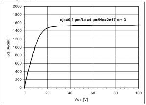
Figure III-2: I-V curve at T=300K (channel depth=0,3  $\mu$ m; channel length=4  $\mu$ m; channel doping level=2  $10^{17}$  cm<sup>-3</sup>, Lintercell=10  $\mu$ m)
