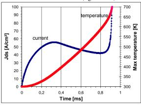
Figure IV-3: Thermal run-away of a silicon current limiting device (same VDS-ramp condition and thermal boundary conditions as for the SiC device figure IV-1).
