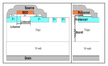
Figure II-1: Vertical cut of the device and its guard rings peripheral protection (the channel length 'Lchannel' and the intercell length 'Lintercell' are noted).
