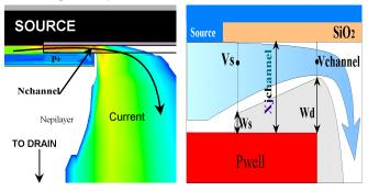
Figure III-3: Left picture: 2D mapping of the current inside the device near the channel region. Right picture: simplified current path in the channel.
