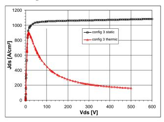
Figure IV-5: Comparison of the static I-V characteristic and electrothermal transient behavior (same structure as figure IV-4).
