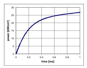
Figure IV-2: Average power versus time (Same conditions as figure IV-1).
