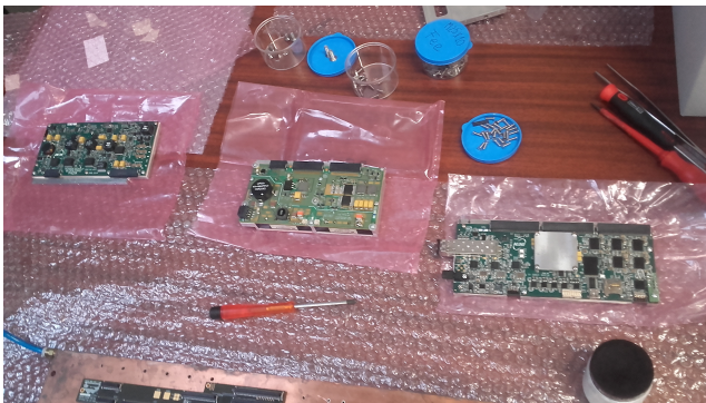
Figure 5: from left to right : Block card, Power Supply, Half Bridge
