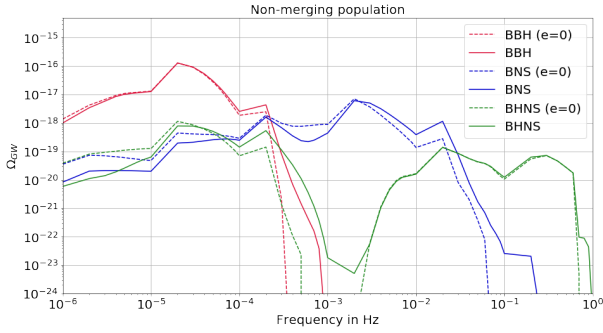
Figure 4: Energy density from binaries which do not merge in a Hubble time including the seven first mode of emission. The solid lines describe the energy densities for each types of binaries with eccentricity evolution while the red dashed one represents the BBH contribution with e = 0 .
