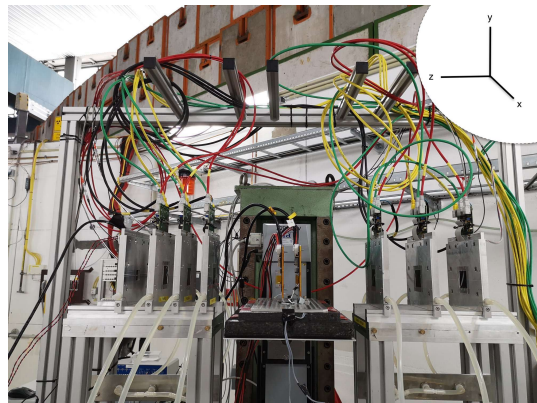
Figure 4: Image of testbeam setup at DESY. Telescope planes are fixed along the beam-z-axis while the DUTs can move upward/downward on the y-axis, inward/outward on the x-axis.
