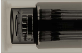
Figure 5: Scanner image of the detector by an X-ray tomography
