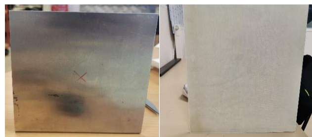
Figure 13: Metallic ground plane and the dielectric substrate
