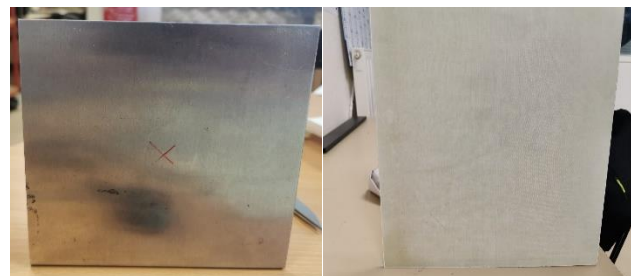
Figure 13: Metallic ground plane and the dielectric substrate
