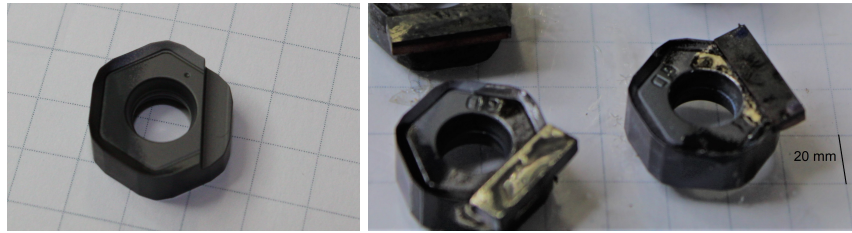
(a) Cutted carbide insert over a 20 mm squares paper (insert manufacturing step 1)
