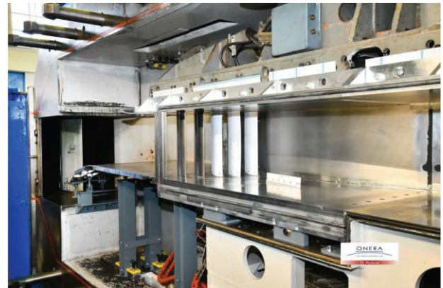
Figure 3 : Overview of the experimental mock-up integration in S3MA wind-tunnel
