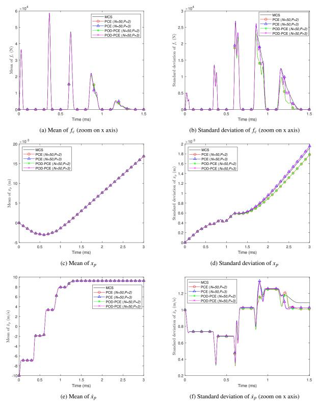
Fig. 7: Time-dependent statistical moments of the stochastic responses for the multiple impact oscillator: MCS was performed using  $N_{\text{MCS}} = 10^4$  model evaluations
