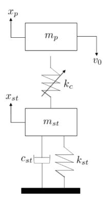
Fig. 1: 2-DOF nonlinear impact dynamic oscillator
