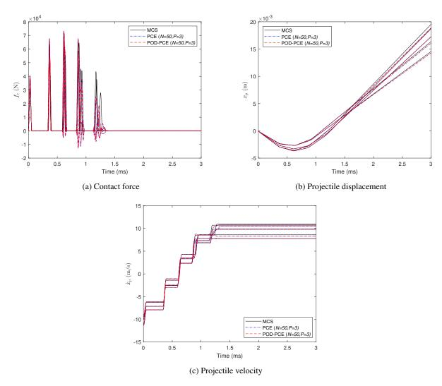
Fig. 9: Comparison of responses for the multiple impact oscillator at 5 samples:  $m_p \in \{342.71, 292.84, 365.62, 310.35, 373.82\}$ g,  $k_c \in \{13.97, 13.87, 14.61, 14.23, 13.63\} \times 10^3 \mathrm{MN \, m^{-3/2}}, v_0 \in -\{11.32, 9.51, 9.96, 9.11, 10.95\}$ ms<sup>-1</sup>
