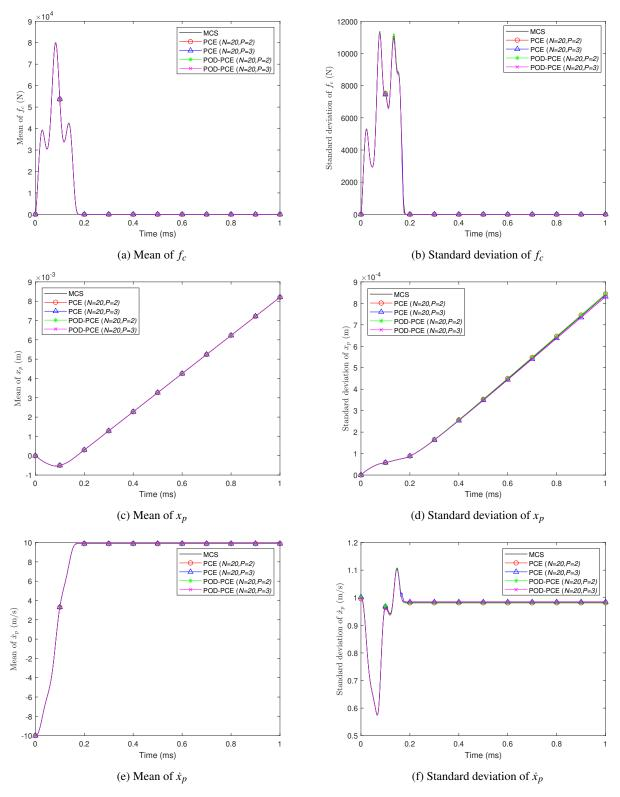
Fig. 3: Time-dependent statistical moments of the stochastic response quantities for the single impact oscillator: MCS was performed using  $N_{\text{MCS}} = 10^4$  model evaluations
