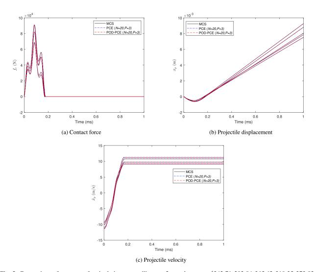
Fig. 5: Comparison of responses for single impact oscillator at 5 samples:  $m_p \in \{342.71, 292.84, 365.62, 310.35, 373.82\}$ g,  $k_c \in \{13.97, 13.87, 14.61, 14.23, 13.63\} \times 10^3 \text{MN m}^{-3/2}, v_0 \in -\{11.32, 9.51, 9.96, 9.11, 10.95\}$ m s<sup>-1</sup>
