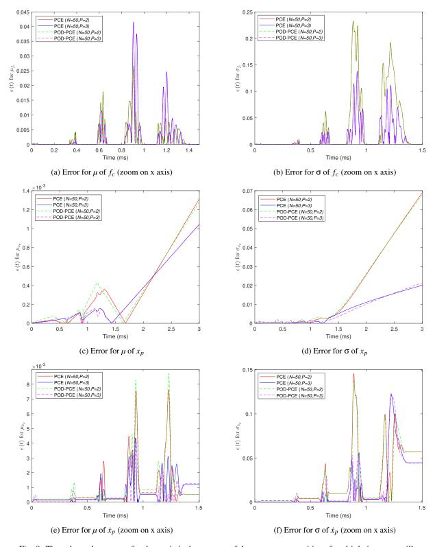
Fig. 8: Time-dependent errors for the statistical moments of the response quantities of multiple impact oscillator
