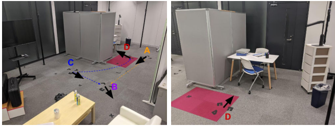
Fig. 4: Environment within the motion capture system with poses A, B, C, D and paths illustrated. Each black arrow is the looking direction of the camera for each pose.
