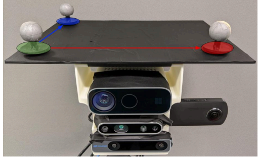
Fig. 1: 3D printed support holding cameras and markers used by the motion capture system
