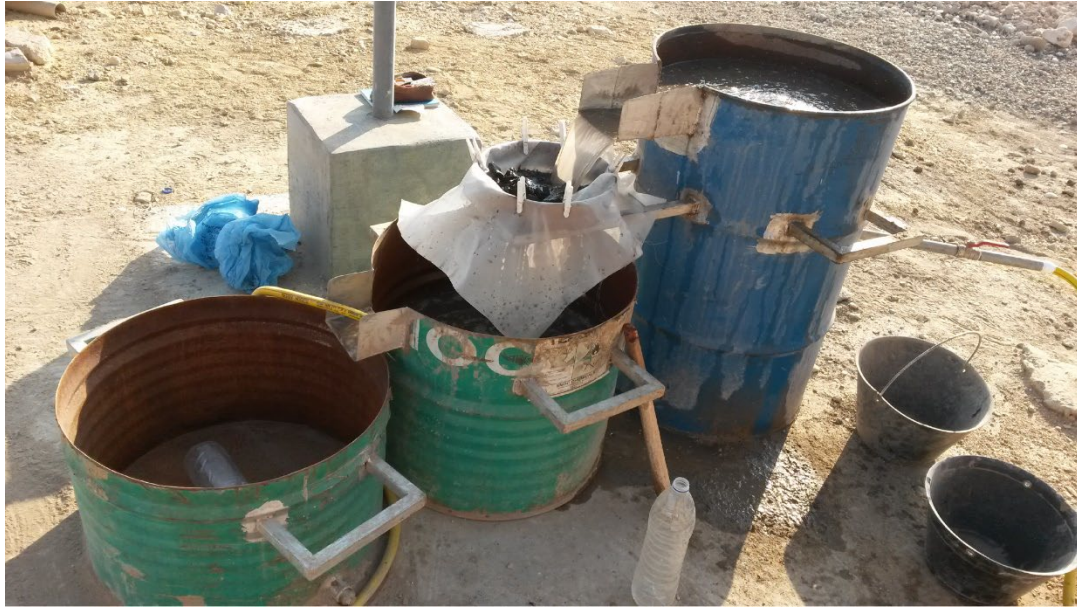
Figure 5. The flotation machine used at Qalhāt constructed from empty oil drums. The main flotation tank to the right (blue) and two decantation tanks to the left (green).
