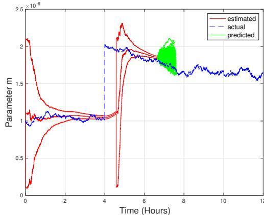
Figure 14: **Prediction scenario 4:** Estimated and predicted trajectories of parameter  $m$  when taken as random following a normal distribution with mean into the estimated uncertainty interval (only 10 predicted trajectories of  $m$  are shown for a better readability)
