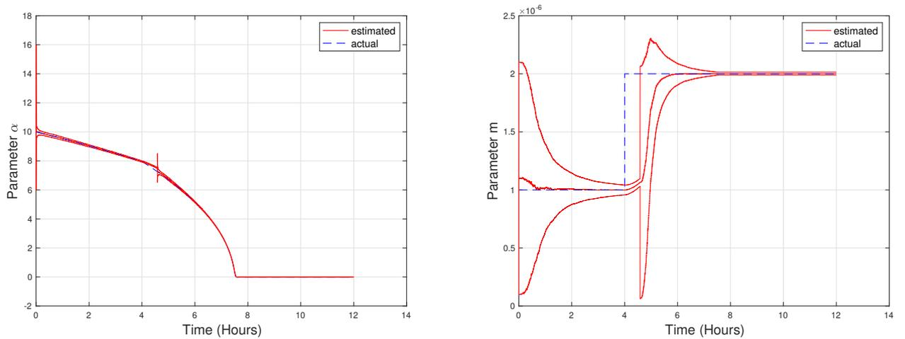
Figure 6: **Estimation scenario:** the parameters  $\alpha$ ,  $m$  and their associated uncertainty intervals are estimated along the whole useful life of a given friction drive. After detection of an abrupt change on  $m$ , which is not considered within the initial model, the EKF observer is re-started with a new matrix  $P_{0|0}$  at around 4.3 hours.
