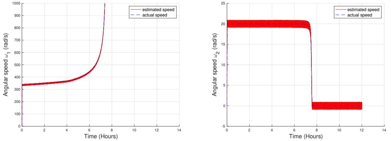
Figure 5: **Estimation scenario:** the angular speeds  $\omega_1$  and  $\omega_2$  (in rad/s) are estimated along the whole useful life of a given friction drive by using noisy measurements. The system lifetime is less than 8 hours, and  $\omega_2 = 0$  after reaching the maximal deterioration.
