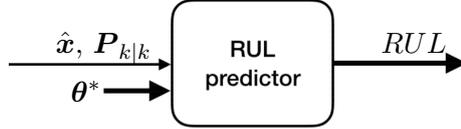
Figure 2: RUL predictor system. The inputs are the estimated deterioration state, its uncertainties and a decision vector  $\boldsymbol{\theta}^*$  concerning desired (or expected) future operation conditions. The output concerns the predicted RUL distribution.
