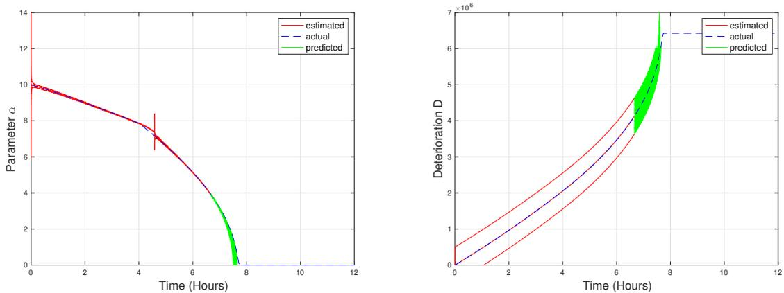
Figure 15: **Prediction scenario 4:** Deterioration ( $\alpha$  and  $D$ ) with correction of the estimation process when  $m$  is taken as random following a normal distribution with mean into the estimated uncertainty interval (only 10 predicted trajectories of  $m$  are shown for a better readability)
