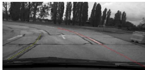
Fig. 1. Example of a disturbed detection due to a severely degraded infrastructure (Revilloud et al 2016 b)
