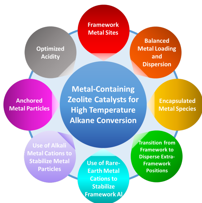
Figure 2. Strategies for improving the performance of metal-containing zeolites catalysts for high temperature alkane conversion.
