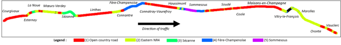
Fig. 4. The NR4 broken center line segmented into 5 replacement areas
