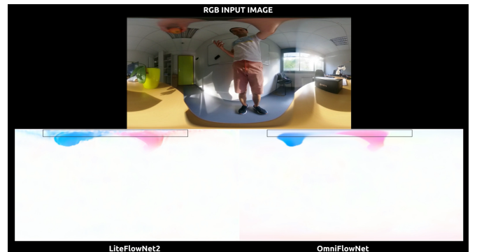
Fig. 9. Apple 1 case: RGB input image (top) and optical flow computed by LiteFlowNet2 (bottom-left) and OmniFlowNet (bottom-right). OmniFlowNet better estimates the optical flow in the top polar region is better. The arm is smoother.
