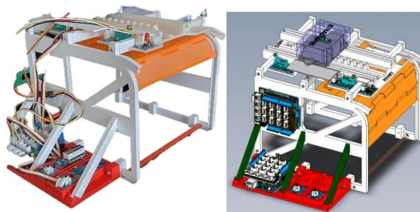
Fig. 10. Scale HOME I/O garage door model
