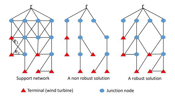
Fig. 1. Support network and solutions on a grid  $4 \times 4$
