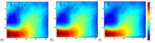
Figure 5. Maps of mean spray density under non-reactive conditions for phase 0° with filter size of a) 25x25 b) 51x51 c) 101x101. Scale in mm
