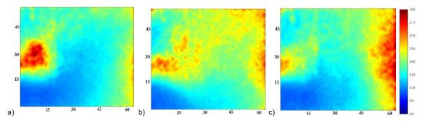
**Figure 9.** Maps of mean nearest-neighbour inter-droplet distance under non-reactive conditions with filter size of 51x51 pixels for phases at a) 0° b) 135° c) 270°. Scale in mm
