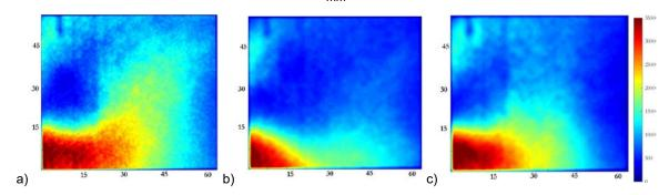
**Figure 8.** Maps of mean spray density (number of droplets per cm²) under non-reactive conditions for phase at a)0° b)135° c) 270°. Scale in mm.
