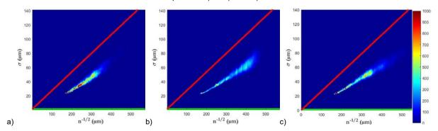
**Figure 11**. Evolution of the standard deviation of nearest-neighbour inter-droplet distance according to the inverse square-root of mean density for phase at a) 0° b) 135° c) 270°
