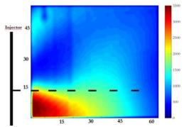
Figure 7. Map of mean spray density (number of droplets per cm²) under non-reactive conditions for stationary study. Scale in
