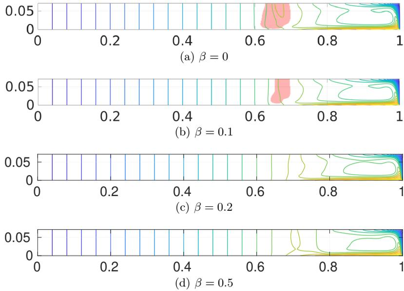
Figure 9: Evolution of the azimuthal velocity  $U_\theta$  for the base flow for increasing  $\beta$ ,  $Re = 18620$  and  $G=1/14$ . 21 equispaced levels in  $[0 - 1]$ . Translucent red patches represent overshoot areas, i.e locations where  $U_\theta \geq 1.01 r$ .
