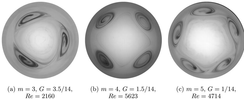
Figure 2: Instability patterns breaking the axisymmetry of the flow. Photograph taken from above (ink visualisation) in our experimental set-up. From left to right : modes  $m = 3, 4$  and  $5$  obtained for different aspect ratios and different values of  $Re$  above the effective  $Re_c$ .
