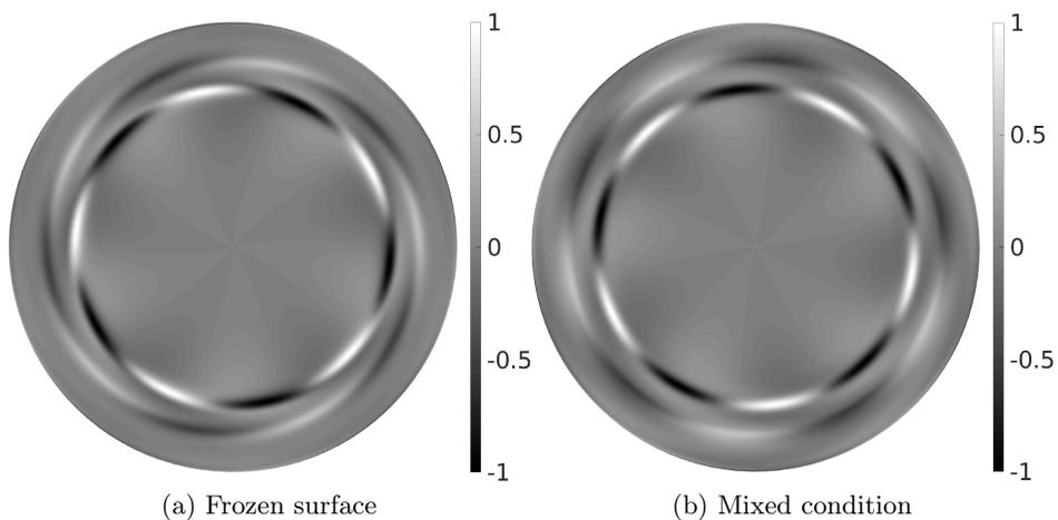
Figure 20: Vorticity  $\omega_z(r, \theta)$  at the fluid interface (normalised by its maximum) for the least stable eigenmode  $m=5$  at  $Re=18620$ . a) frozen surface, b) mixed condition. The mixed condition corresponds to a frozen surface condition for the base flow, and free surface condition for the perturbation field.
