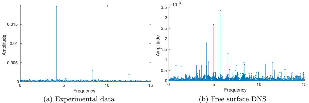
Figure 7: Comparison of frequency amplitude spectra for  $u_\theta(t)$  measured at  $r = 0.76$ ,  $z = 0.8G$ , for the saturated  $m=5$  regime at  $Re = 18620$ . Left: experimental, maximum peak at  $f = 4.15$ . Right: DNS with free surface condition, same parameters. The frequencies are not normalized by the azimuthal wavenumber.
