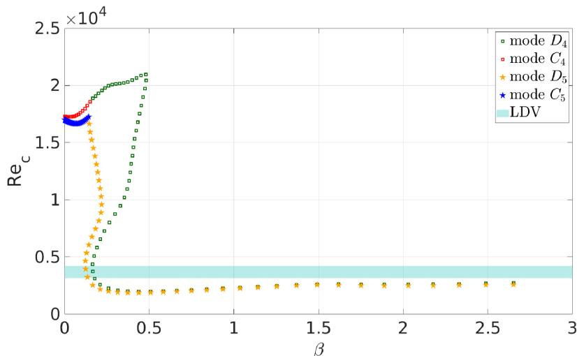
Figure 10: Neutral curve  $Re_c(\beta)$  estimated from LSA for  $G=1/14$  and for the modes  $m=4$  (squares) and  $m=5$  (stars). The blue strip corresponds to the experimental value of  $Re_c$ , independent of the model based on  $\beta$ . The thickness of the strip is based on lower and upper bounds for  $Re_c$  from Table 1.
