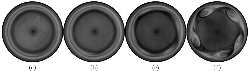
Figure 3: Instability growth for a  $m = 5$  mode for a water + Kalliroscope mixture initially at rest.  $G=1/14$ , Reynolds number  $Re=16\ 550$ . 3a)  $t = 52s$ , 3b)  $t = 60s$ , 3c)  $t = 71s$ , 3d)  $t = 99s$ .
