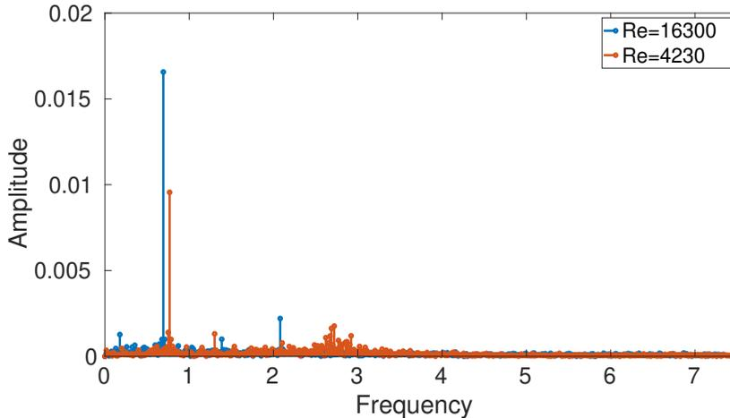
Figure 4: Experimental frequency amplitude spectrum of azimuthal velocity component measured at  $r=0.76$ ,  $z=0.9G$ , for the saturated  $m=5$  regime at  $Re=4230$  and  $Re=16300$ . The maximum peak amplitudes correspond to  $f=0.76$  and  $f=0.73$  respectively.
