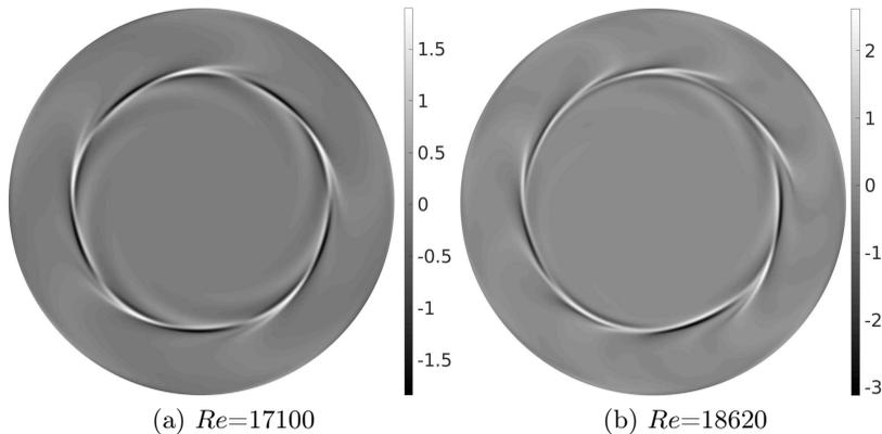
Figure 6: DNS axial vorticity fluctuation for the free surface condition,  $Re=17100$  (slightly above  $Re_c$  (6a), and  $Re=18620$  (6b). With the increase of  $Re$ , the mode  $m=5$  selected at  $Re_c$  evolves into a modulated  $m=7$  pattern.
