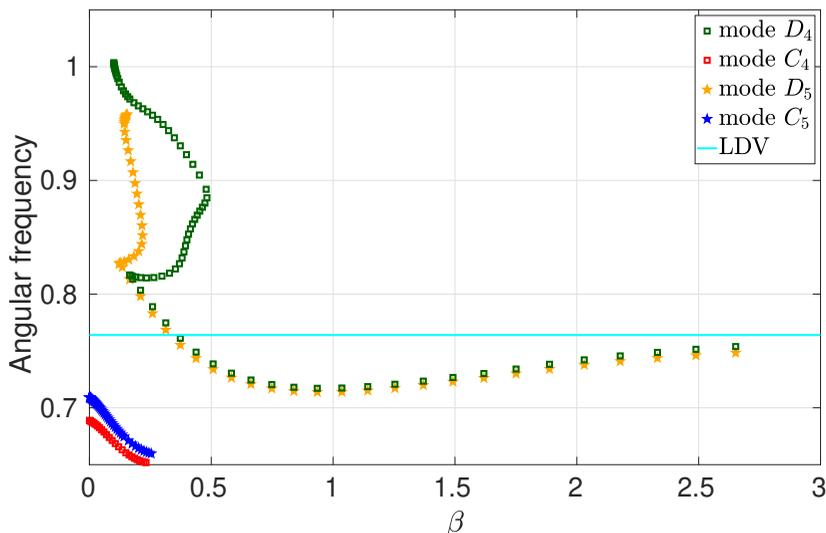
Figure 13: Angular frequency of the pattern  $-\mathcal{I}m(\lambda)/m$  at  $Re = Re_c(\beta)$  for  $G=1/14$ , obtained using LSA for the modes  $m=4$  (squares) and  $m=5$  (stars). The blue strip corresponds to the experimental value obtained using LDV (cf Table 1).
