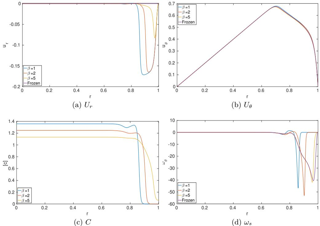
Figure 15: Comparison of several fields of the base flow at the surface, for few values of  $\beta$ , at  $Re=18620$ . 15a) radial velocity  $U_r$ , 15b) azimuthal velocity  $U_\theta$ , 15c) pollutant concentration  $C$ , 15d) azimuthal vorticity  $\omega_s$ . The results for the frozen surface condition are also included in the figures.
