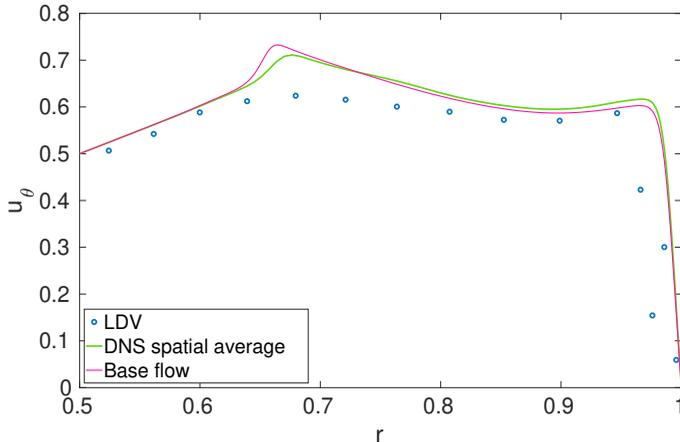
Figure 5: Velocity profiles of  $u_\theta(r)$  below the free surface ( $z = 0.8G$ ) for  $G=1/14$  and  $Re = 18620$ . Comparison between the base flow, spatially averaged DNS and the temporal average for LDV (experiment). LDV acquisition timespan is much larger than the instability period.
