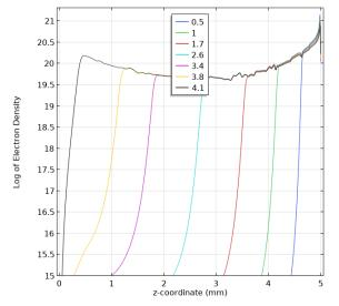
Figure 5: Line graph of the log of the Electron Density Distribution along the symmetry axis for different time steps.
