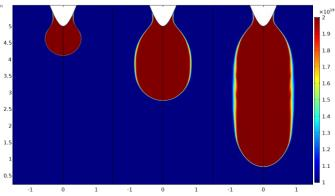
Figure 3: 2D surface plots of electron density profiles of a streamer propagating in a 5 mm air gap at times t = 1.0, 2.5 and 3.9 ns.
