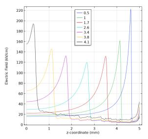
Figure 6: Line graph of Electric Field Distribution along the symmetry axis corresponding to figure 5.
