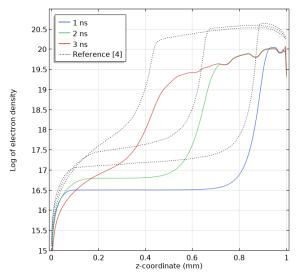
Figure 1: Electron density variation on streamer axis at times t = 1, 2 and 3 ns for our model (solid line) and original work [4] (dotted line).
