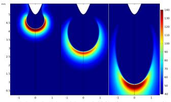
Figure 4: 2D surface plots of electric field distributions corresponding to electron densities in figure 3.
