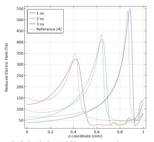
Figure 2: Reduced electric-field variation on the streamer axis corresponding to figure 1.
