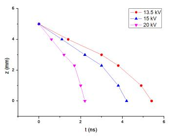
Figure 7: Position of streamer head as a function of time for applied voltages, 13.5 kV, 15 kV and 20 kV in a 5 mm gap.
