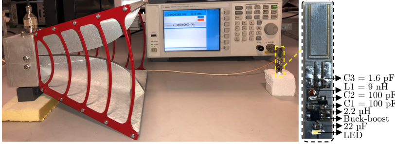
Figure 11: Testbench used to characterize the proposed rectenna driving a LED.
