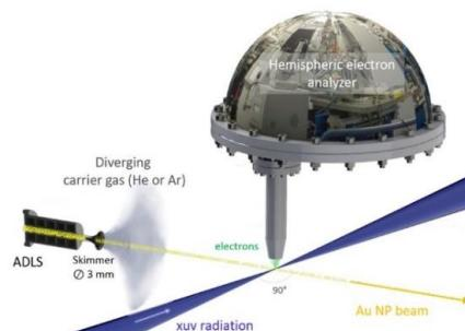
**Figure 1.** An aerosol of AuNPs is created using an atomizer. An aerodynamic lens focuses the AuNP beam to the interaction region with soft X-rays of PLEIADES beamline (Synchrotron SOLEIL).
