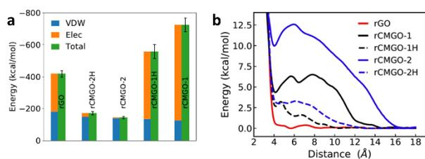
**Figure 5.** a): Average pair interaction energy between water molecules and respective rGO/rCMGO surfaces and right b): PMF energy profile of water molecules with rGO (red), rCMGO-1/rCMGO-1H (black) and rCMGO-2/rCMGO-2H (blue) surfaces. VDW, Elec energies correspond to van der Waals and electrostatic contributions to the total (Total) energies.
