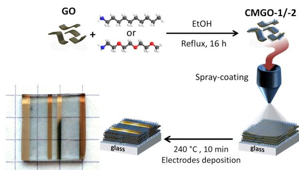
**Figure 1.** Schematic representation of the reaction of GO with either NTEG or decylamine, and device preparation. Bottom-left: photo of the actual sensor (lateral size: 1.2 cm). The underlying square pattern serves to demonstrate the optical transparency of the device.
