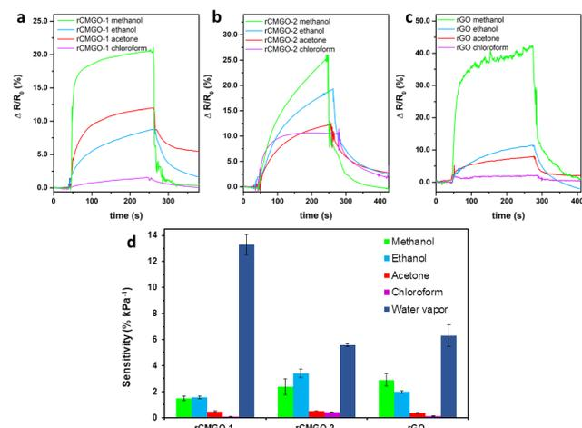
**Figure 4.** Selectivity response in function of time when a) rCMGO-1, b) rCMGO-2 and c) rGO are exposed alternatively to nitrogen and to saturated vapours of methanol (green line), ethanol (blue line), acetone (red line) and chloroform (purple line). d) Sensitivity of the devices (% kPa<sup>-1</sup>) to the same vapours and to humidity (100 % RH) obtained dividing the maximum response to the analytes by its saturation vapor pressure at 20 °C expressed in kPa.
