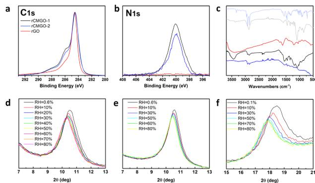
**Figure 2.** XPS spectra of C1s peak (a) and N1s peak (b) of rCMGO-1 (black), rCMGO-2 (blue) and rGO (red). c) FTIR-ATR of CMGO-1 (black), CMGO-2 (blue) and GO (red), decylamine (light blue) and NTEG (gray). Variation of the XRD patterns upon exposure to humidity of the (d) rCMGO-1, (e) rCMGO-2, and (f) rGO films.
