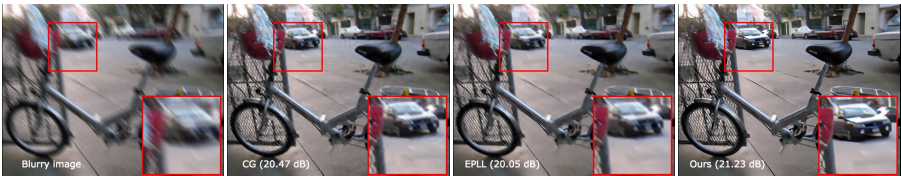
Fig. 7: Non-uniform motion deblurring example with 1% additive Gaussian noise (better seen on a computer screen). The car and the helmet are sharper with our method than in the images produced by our competitors.
