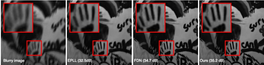
Fig. 4: Comparison of state-of-the-art methods and the proposed LCHQS for one sample of the Levin dataset [23] (better seen on a computer screen). FDN effectively removes the blur but introduces artifacts in flat areas, unlike EPLL and LCHQS.
