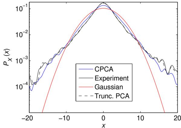
FIG. 10. Probability density functions  $p_X(x)$ , of variable  $X_{129}$ , logarithmic scale. Original data ("Experiment"), PCA truncated to  $m=15$  terms ("Trunc. PCA"), its Gaussian approximation, and CPCA optimum least squares solution with  $N=3$  and  $n_d=3$ ,  $\epsilon_{ovl}^{(129)}=0.1654$ .
