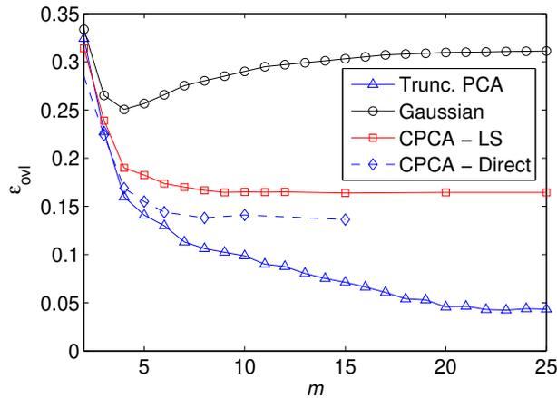
FIG. 13. Minimum error  $\epsilon_{ovi}(N, n_d)$  vs.  $m$  for PCA truncated to  $m=15$  terms ("Trunc. PCA"), its Gaussian approximation, and the CPCA optima obtained by direct optimization and least squares approach over the value of  $N$  for  $n_d=3$ .
