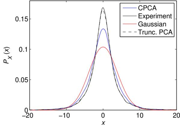
FIG. 9. Probability density functions  $p_X(x)$ , of variable  $X_{129}$ , linear scale. Original data ("Experiment"), PCA truncated to  $m=15$  terms ("Trunc. PCA"), its Gaussian approximation, and CPCA optimum least squares solution with  $N=3$  and  $n_d=3$ ,  $\epsilon_{ovl}^{(129)}=0.1654$ .
