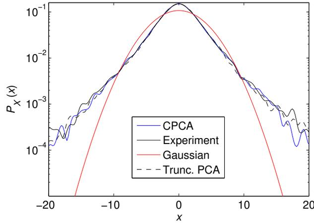
FIG. 6. Probability density functions  $p_X(x)$ , of variable  $X_{157}$ , logarithmic scale. Original data ("Experiment"), PCA truncated to  $m=15$  terms ("Trunc. PCA"), its Gaussian approximation, and CPCA optimum least squares solution with  $N=3$  and  $n_d=3$ ,  $\epsilon_{\text{opt}}^{(157)}=0.0251$ .
