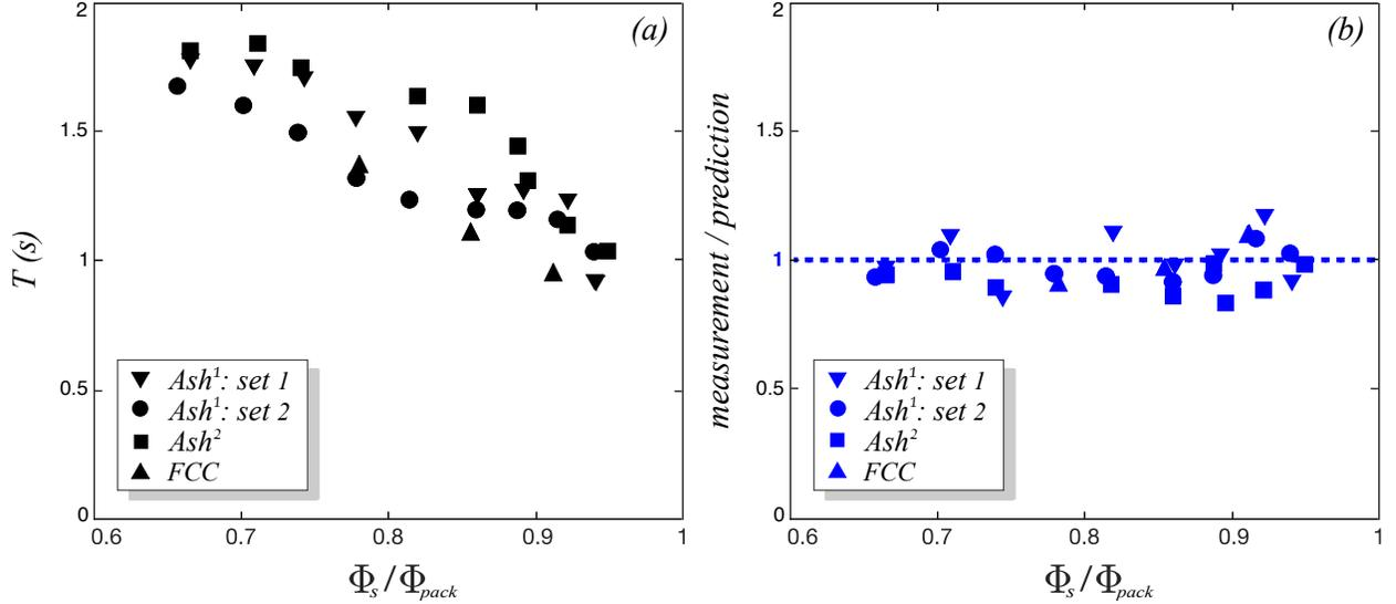
FIG. 6. Assessment of the model regarding the total duration  $T$ . (a) measured values of  $T$  as a function of  $\Phi_s/\Phi_{pack}$ , for all experiments. (b) Ratio between measured values of  $T$  and values predicted by eq (8).
