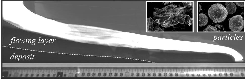
FIG. 2. Picture of the dam-break flow of an expanded suspension of volcanic ash heated at  $180^{\circ}\text{C}$ . Note that the picture is not a pure side view, but taken from a point above the surface. The whitish zone corresponds to the surface the suspension seen in perspective. The two inserts are pictures of volcanic ash (on the left) and FCC particles (on the right).
