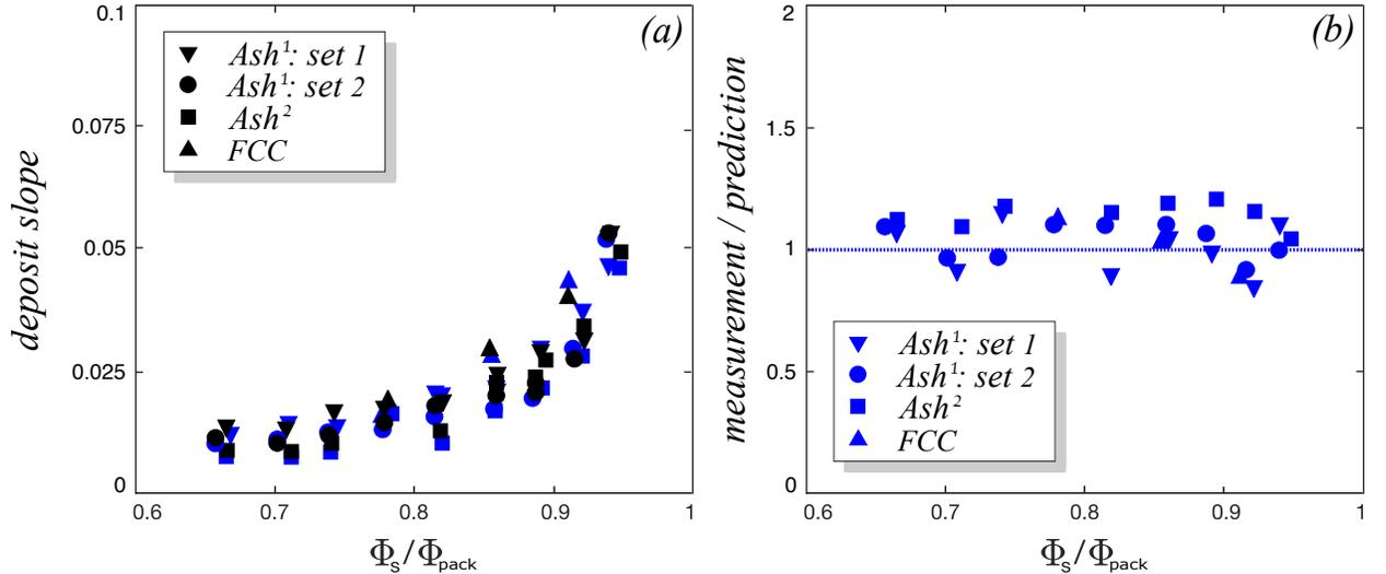
FIG. 5. Assessment of the model regarding the deposit slopes. (a) Measured deposit slopes  $|h_{d\infty}/L|$  (black symbols) and values predicted by eq (6) (blue symbols) as a function of  $\Phi_s/\Phi_{pack}$ , for all experimental cases. (b) Ratio between measured and predicted slopes.
