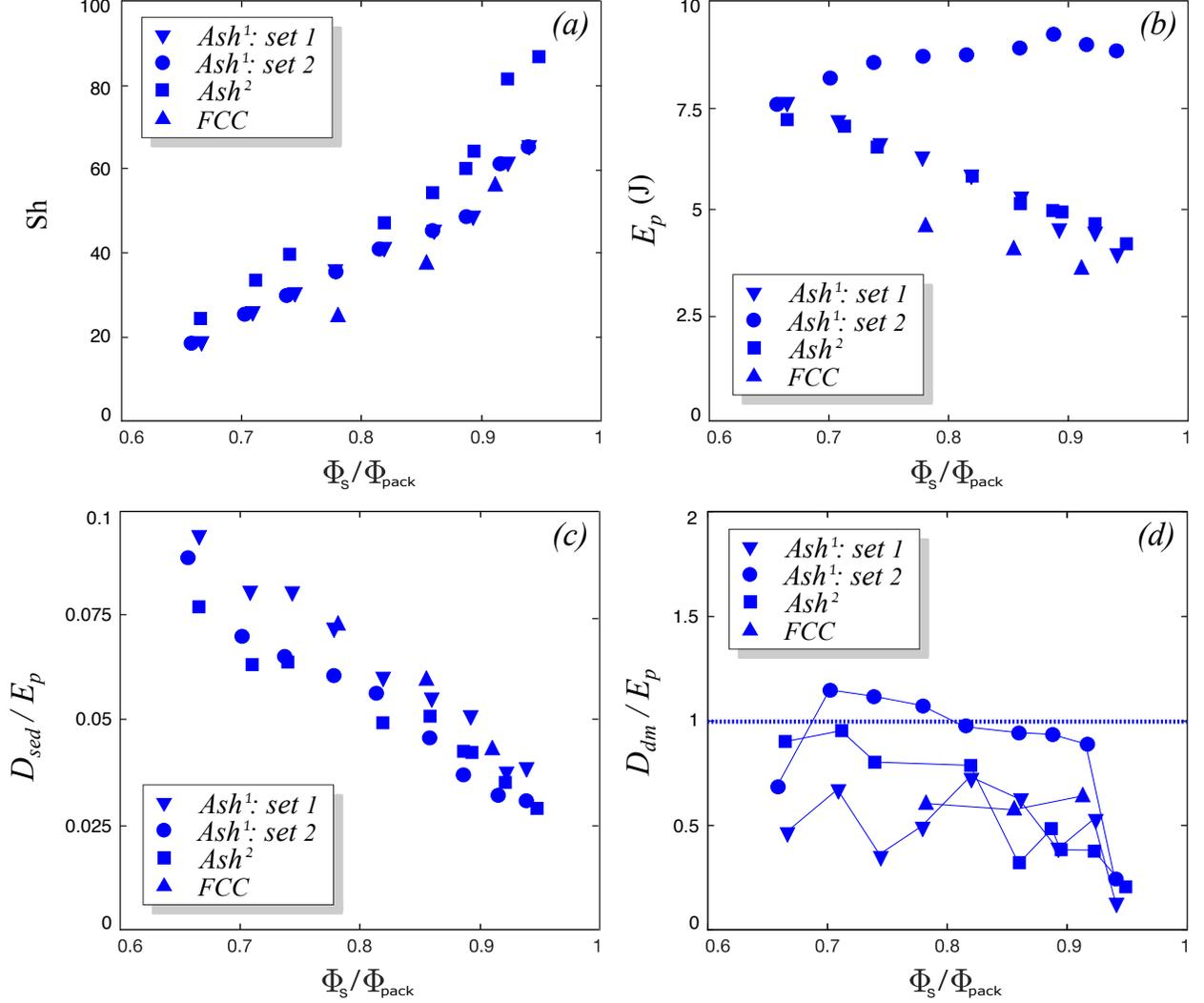
FIG. 7. Analysis of the wall friction  $\tau_p$  and of its contribution to the dissipation from experimental data. (a) Shields number comparing wall friction to particle weight; (b) Potential energy  $E_p$  released during the total flow duration; (c) Energy  $D_{sed}$  dissipated by the sedimentation flow; (d) Energy  $D_{ab}$  lost by dam-break flow due to  $\tau_p$ , calculated under the assumption of a linear longitudinal velocity profile, eq (22).
