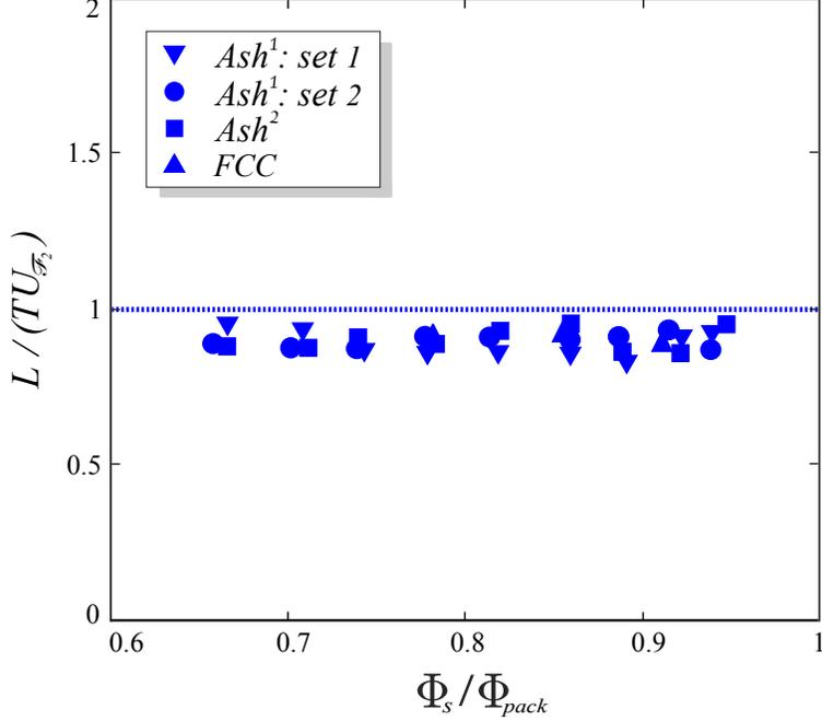
FIG. 3. Experimental ratio between the average front velocity ,  $L/T$ , and the constant velocity of the second phase of the dam-break-flow,  $U_{\mathcal{F}_2}$ , as a function of  $\Phi_s/\Phi_{pack}$ , for all experiments.
