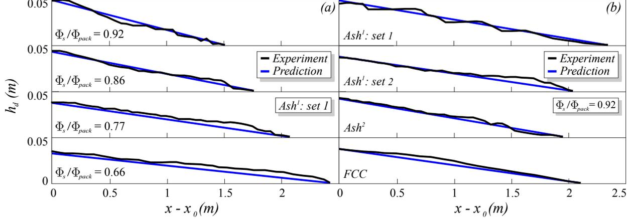
FIG. 4. Profiles of the final deposit within the channel ( $x_0 \leq x \leq L$ ). Black curves, experimental data; blue lines, model prediction. (a)  $Ash^2$  deposits obtained for different values of  $\Phi_s/\Phi_{pack}$ ; (b)  $Ash^1$ ,  $Ash^2$ , and  $FCC$  deposits obtained at a given value of  $\Phi_s/\Phi_{pack}$ .
