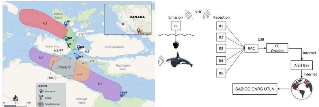
**Figure 1.** Left: Map of the area and the listening range of the 5 hydrophones H1 to H5. Detection zones indicate which hydrophones can record Orca calls in a given area, w.r.t. thirty years of observations by Orcalab. Right: Representation of the data acquisition, from recording until storage at Toulon.
