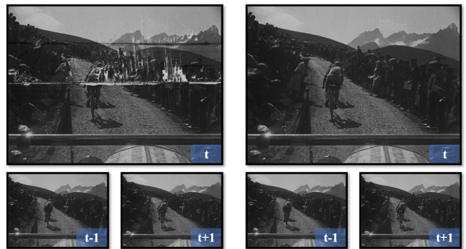
(a) Three consecutive frames with line scratches and blotches in the central one
