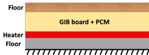
Figure 13 Underfloor heating system layout [17].
