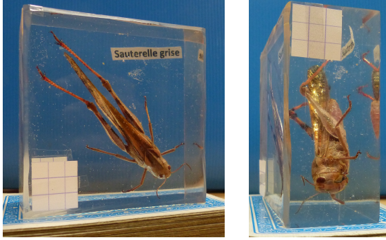
Figure 15: Two real images of a grasshopper cast in a box-shaped block of resin. The small grid glued on each side allows us to estimate the camera pose and the position of the planar interface.
