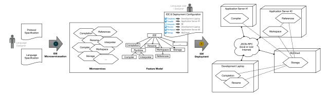
Figure 3. Approach overview, with the two main steps: ① IDE microservicesation and ② IDE deployment
