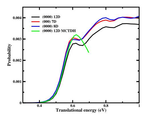
FIG. 2. The calculated  $J_{tot} = 0$  reaction probabilities for the H+CH<sub>4</sub>(0000)  $\rightarrow$  H<sub>2</sub>+CH<sub>3</sub> as a function of translational energy for different kinds of methods: in black our new 12D calculations, in red model with 7 dimensions, in blue with 8 dimensions, in green calculations with MCTDH with a slightly different PES.
