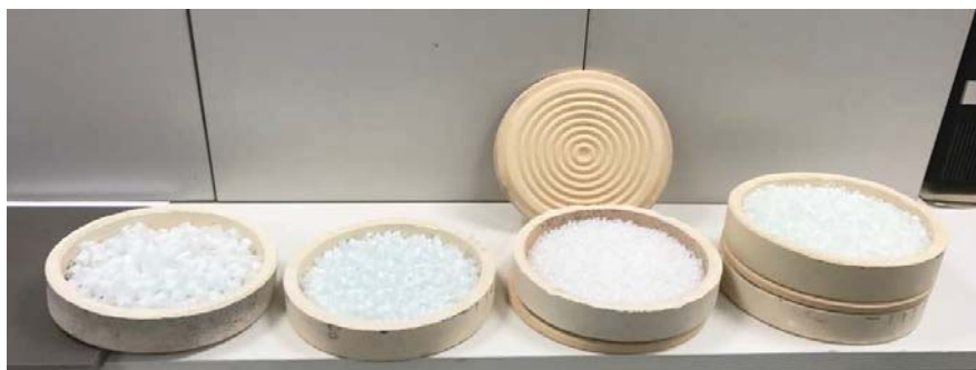
Fig. 2 glass Raschig rings coated with a thin film of TiO 2
