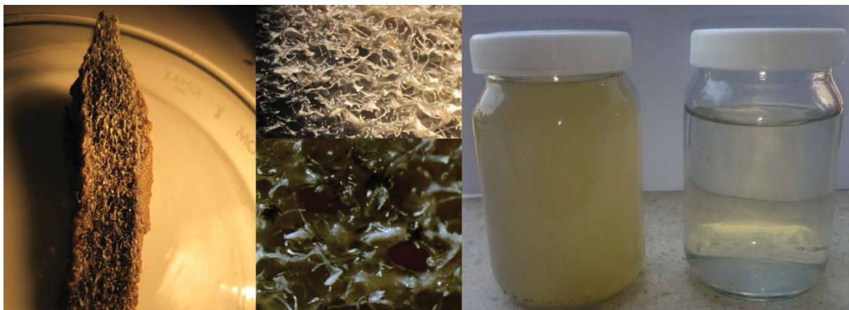
Figure 7 Substratum with biofilm (left) Input and output of the bioreactor (right).
