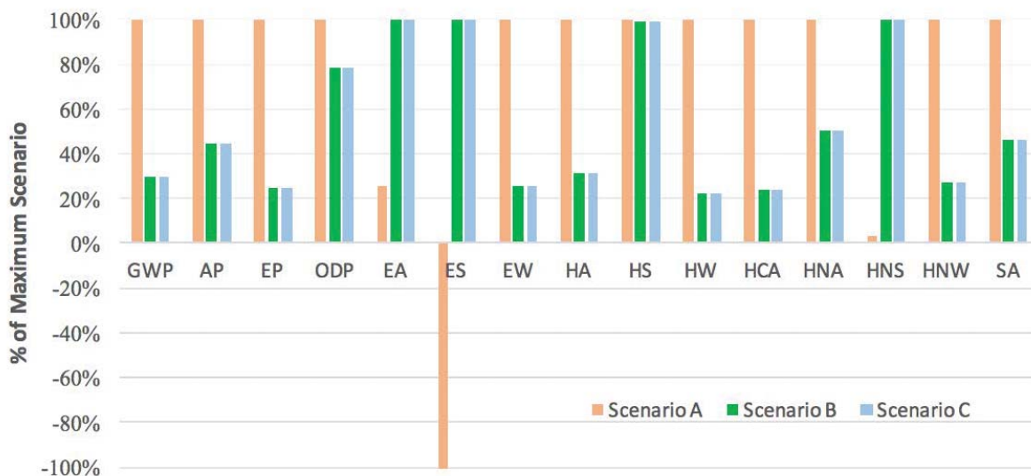
Figure 3. Environmental impact of each scenario; GWP -global warming air, AP -acidification air, EP -eutrophication, ODP -ozone depletion air, EA -ecotoxicity air, ES -ecotoxicity soil, EW -ecotoxicity water, HA -human health cancer air, HS -human health cancer soil, HW -human health cancer water, HCA -human health criteria air, HNA -human health non cancer air, HNS -human health non cancer soil, HNW -human health non cancer water, SA -smog air.
