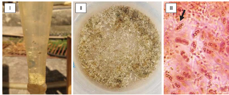
Figure 3. (I) Settling test of R2-packed effluent (HRT = 6h) after 30 minutes, with white solids at the bottom of the Imhoff cone; (II) white precipitate present in the R2-packed effluent; (III) microscopic image of purple bacteria in R2-packed biomass (HRT = 4h), emphasizing intracellular elemental sulphur.
