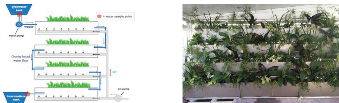
Fig. 1. Schematic overview of the VertECO unit (left). Demonstration unit at the hotel (right).
