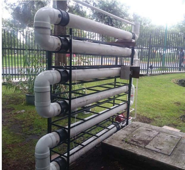
Figure 1. Tubular biological reactor
