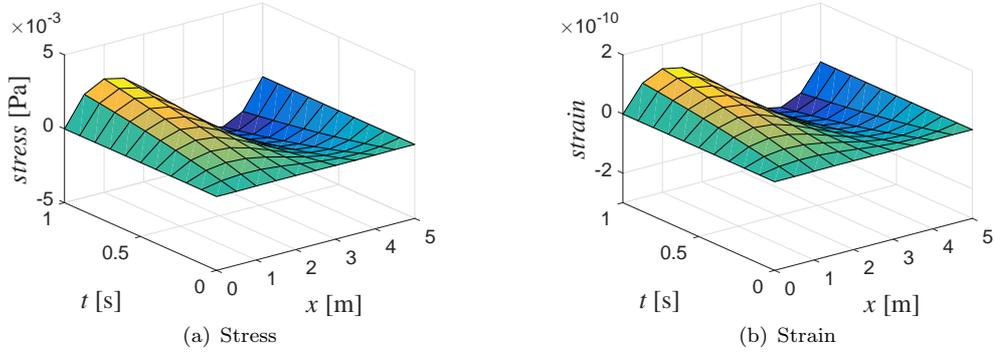
Figure 9: Stress and strain of concrete viscoelastic column.
