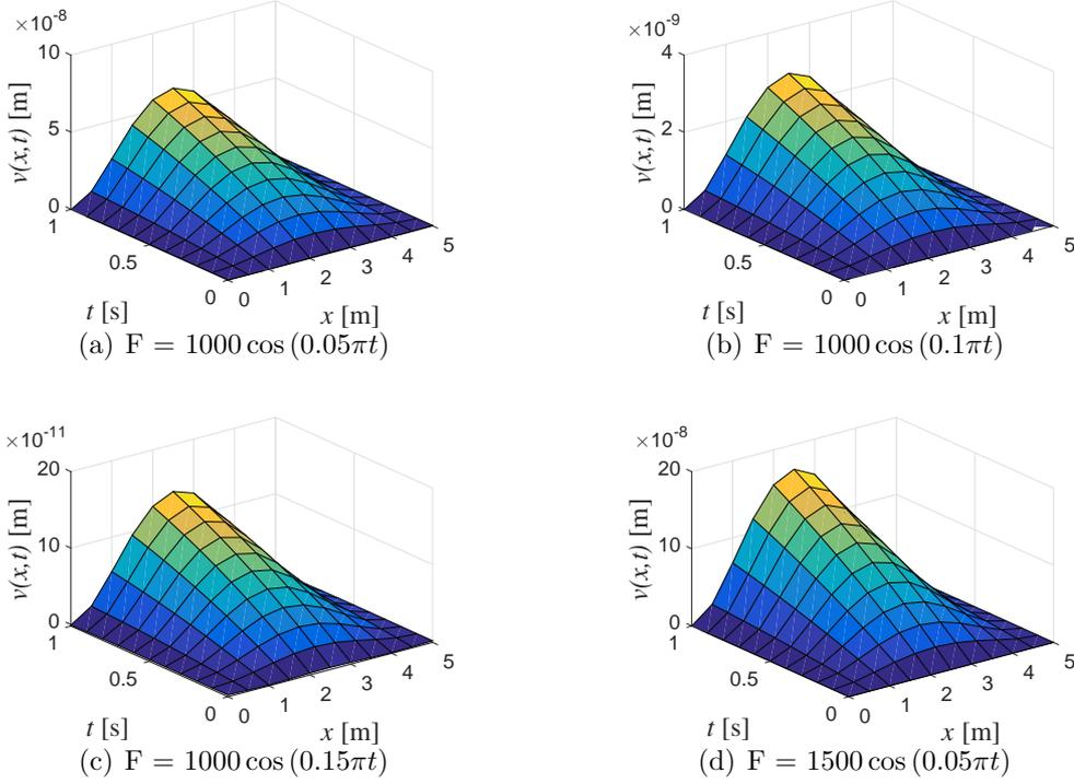
Figure 7: Transverse displacement of viscoelastic column under different harmonic loads: (a)  $F = 1000 \cos(0.05\pi t)$ , (b)  $F = 1000 \cos(0.1\pi t)$ , (c)  $F = 1000 \cos(0.15\pi t)$ , (d)  $F = 1500 \cos(0.05\pi t)$
