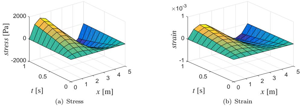
Figure 10: Stress and strain of polymer viscoelastic column.
