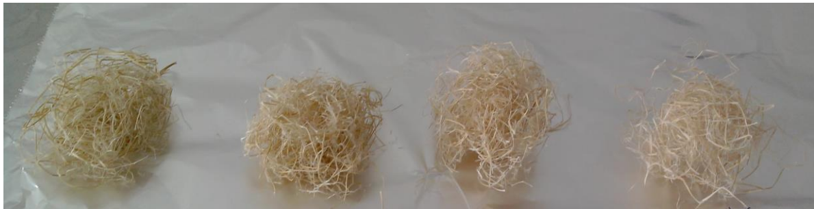
Figure 8. Photograph of the treated fibres. (a) NaOH treated fibres, (b) xylanase treated fibres, (c) pectinase treated fibres and (d) laccase treated fibres
