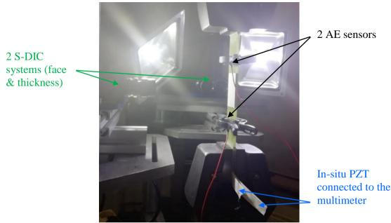
Figure 3: The multi-instrumented test
